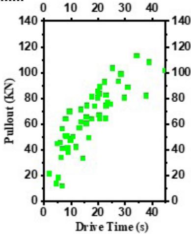
**Fig.16.** Pullout load-displacement with drive time for a)  $D = 34$  mm, b)  $D = 36$  mm and c)  $D = 38$  mm
