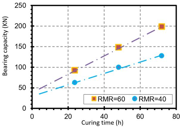
**Fig.13.** Pull-out bearing capacity with Curing Time
