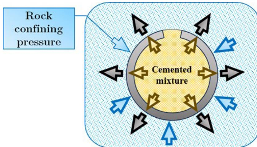
*Fig.5. Radial confining pressure of rock mass*
