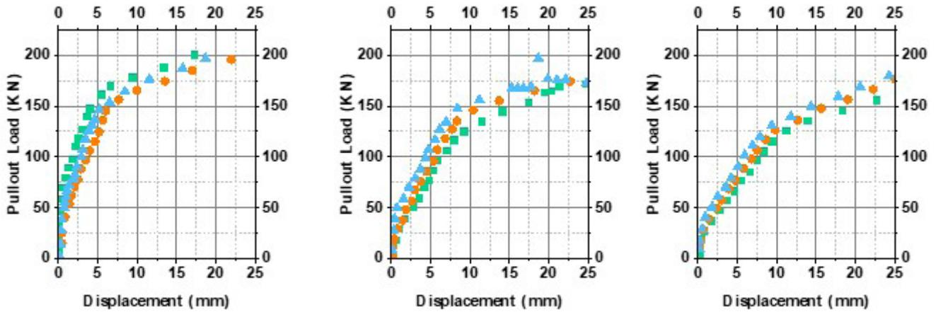
**Figure 7.** a) Pullout load-displacement for RMR=40; b) Pullout load-displacement for RMR=60; c) Pullout load-displacement for RMR=80
