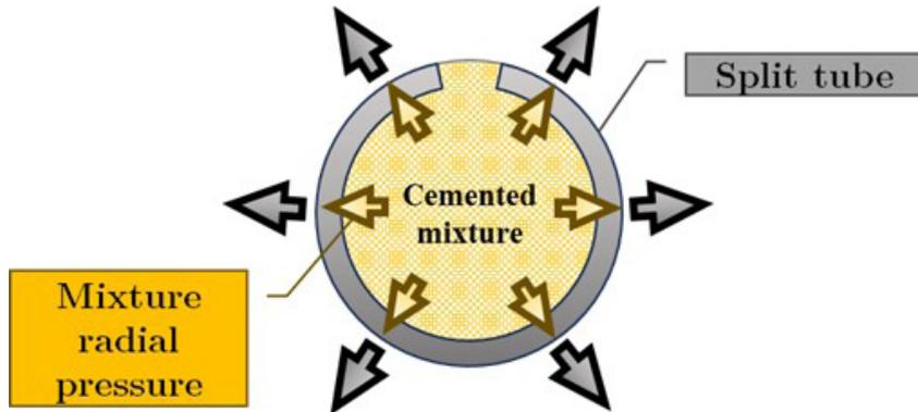
*Fig.4. Radial pressure of cementation mixture.*
