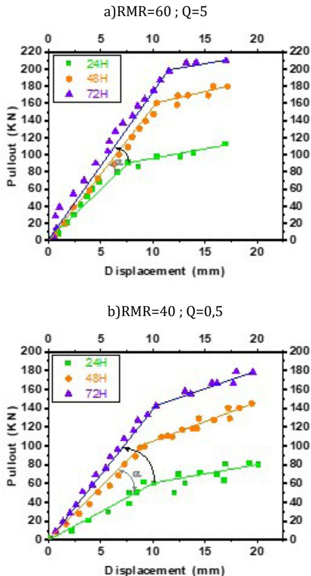
**Fig. 12.** Pull-out bearing capacity with lengths ranging a) RMR=60 b) RMR=40
