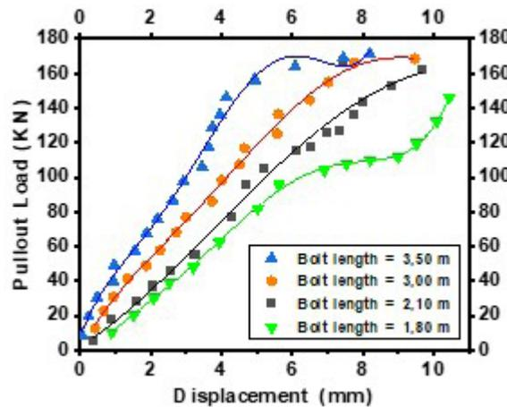
**Fig. 9.** Pullout load-displacement with lengths ranging for a) RMR=40 b) RMR=60 and c) RMR=80
