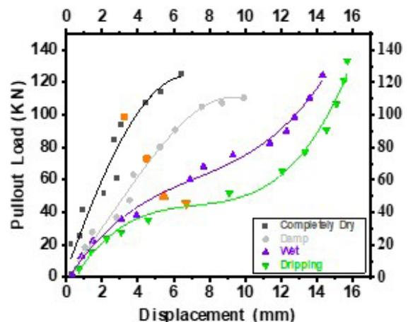
**Fig.14.** Pullout load-displacement with groundwater factor for RMR=60
