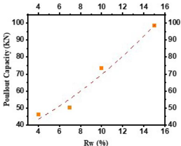
**Fig.15.** Pull-out bearing capacity with groundwater factor for RMR=60
