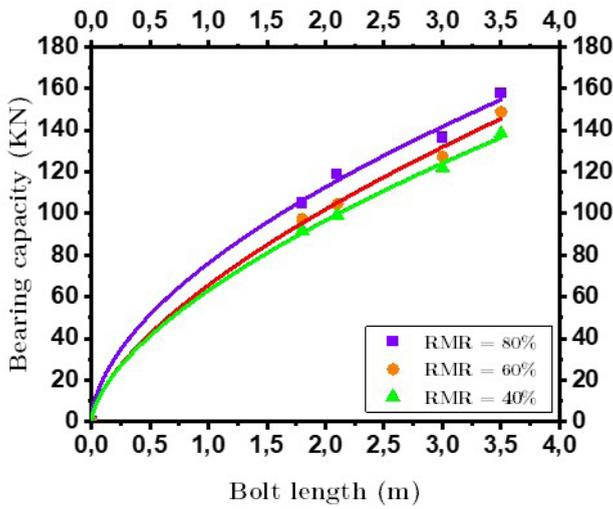
**Fig. 10.** Pull-out bearing capacity with lengths ranging
