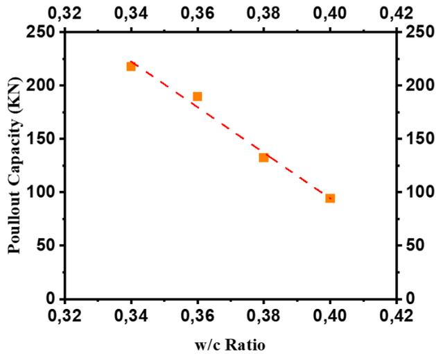
**Fig.18.** Pull-out bearing capacity with WCR ratio (RMR=60; Curing time=28 Days)
