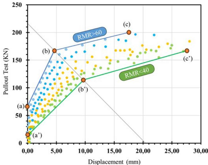
**Fig.8.** Pullout load-displacement for RMR=40, RMR=60 and RMR=80
