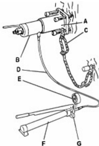
**Fig.3.** Pull-out test setup (A: Charging case - B: Jack - C: Safety chain - D: Hydraulic hose - E: Manometer - F: Hand pump - G: Valve)
