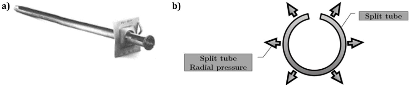
**Fig.2.** a) Friction bolt / Split set (Hoek, 1993) b) Radial pressure of the friction bolt
