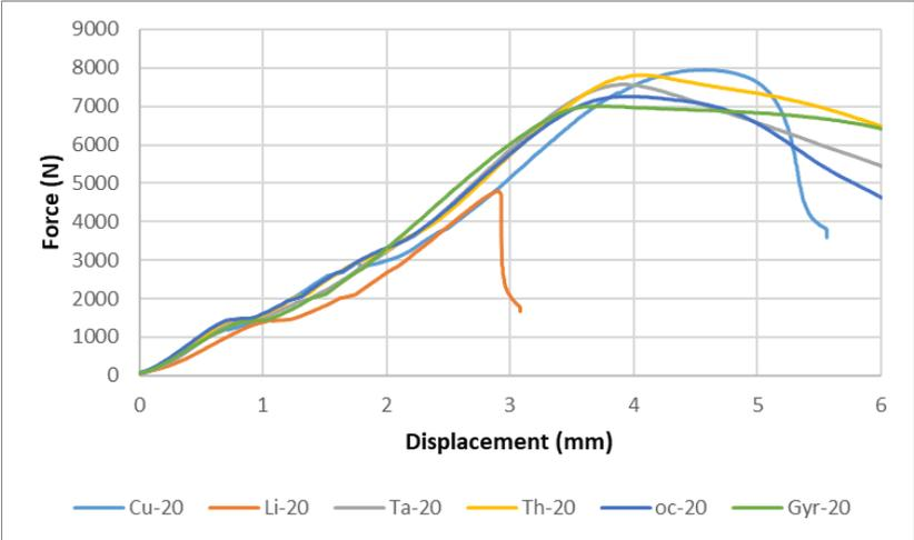
**Figure 4.** Force-displacement curves obtained from the samples with a 20% infill density
