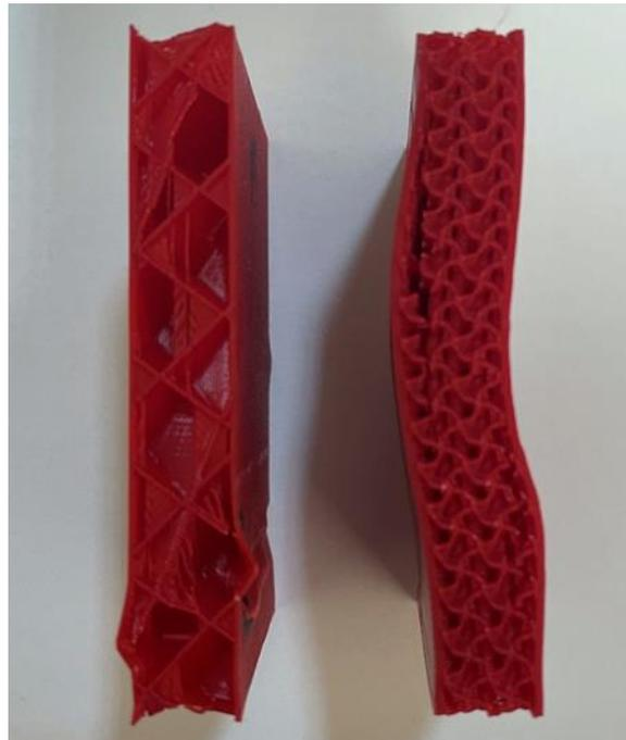
**Figure 3.** Unacceptable and acceptable types of damages
