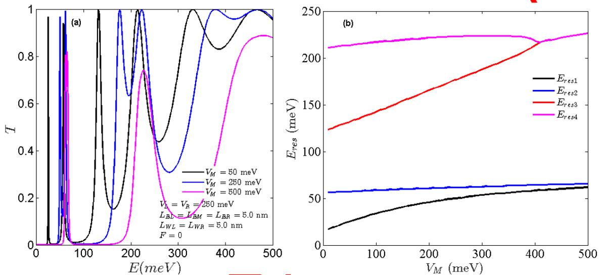
**Figure 3.** (color online) **a)** The variation of the transition probability with respect to the incident electron energy for three different medium potential barrier heights ( $V_M = 50, 250,$  and  $500$  meV). **b)** The graph of the resonance energy change depending on the medium potential barrier height. System parameters were chosen as  $L_{WL} = L_{WR} = 5$  nm,  $V_L = V_R = 250$  meV, and  $F = 0.0$
