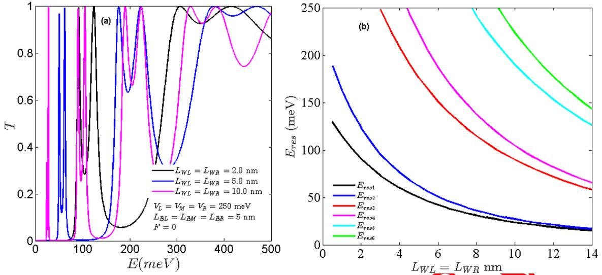
**Figure 6.** (color online) **a)** The variation of the transition probability according to the incident electron energy for three different well widths ( $L_{WL} = L_{WR} = 2.0, 5.0$  and  $10.0$  nm). **b)** The graph of the resonance energy variation depending on the well widths. System parameters were chosen as  $L_{BL} = L_{BM} = L_{BR} = 5$  nm,  $V_L = V_M = V_R = 250$  meV, and  $F = 0.0$
