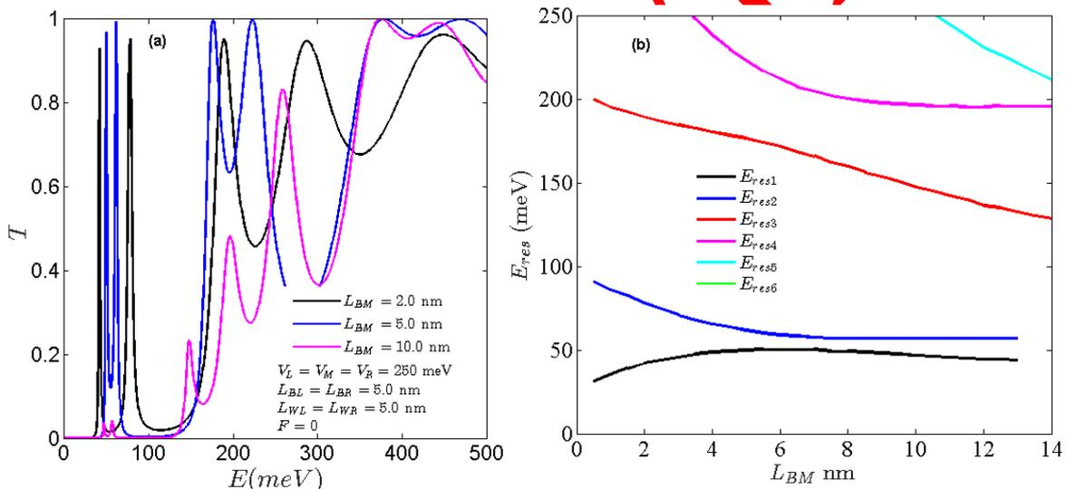
**Figure 5. a).** The variation of the transition probability with respect to the incident electron energy for three medium barrier widths ( $L_{BM}=2.0, 5.0,$  and  $10.0$  nm). **b)** The graph of change of resonance energy depending on the middle barrier width. The system parameters were chosen as  $L_{BL}=L_{BR}=5$  nm,  $L_{WL}=L_{WR}=5$  nm,  $V_L=V_M=V_R=250$  meV, and  $F=0.0$
