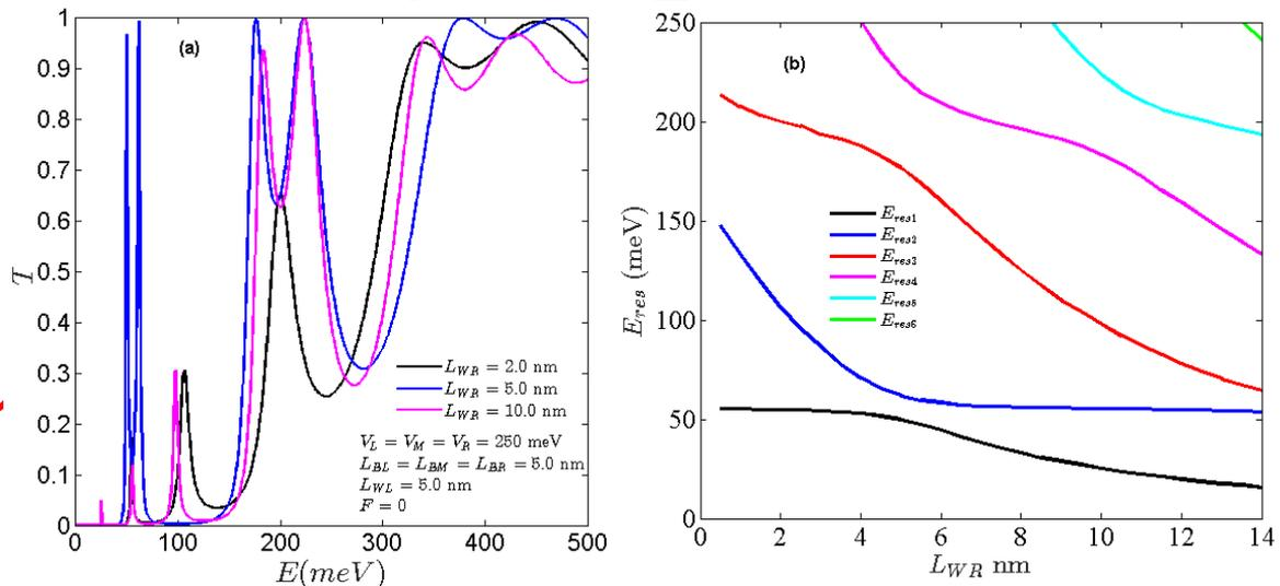
**Figure 7.** (color online) **a)** The variation of the transition probability for three different right well widths ( $L_{WR} = 2.0, 5.0$ , and  $10.0$  nm) with respect to the incident electron energy. **b)** Graph of change of resonance energy depending on the right well width. System parameters were chosen as  $L_{WL} = 5$  nm,  $L_{BL} = L_{BM} = L_{BR} = 5$  nm,  $V_L = V_M = V_R = 250$  meV, and  $F = 0.0$
