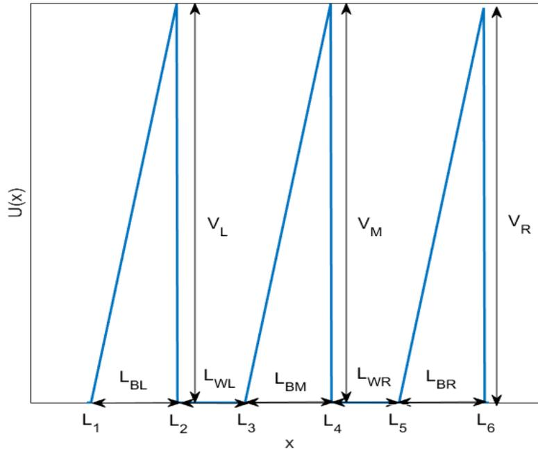
Figure 1. Sawtooth triple barrier potential structure
