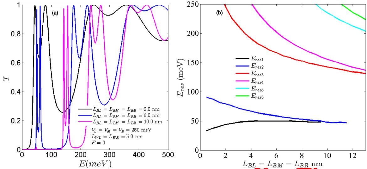
**Figure 4.** (color online) **a)** The variation of the transition probability according to the incident electron energy for three different barrier widths ( $L_{BL}=L_{BM}=L_{BR}=2.0, 5.0$  ve  $10.0$  nm). **b)** The graphs of the resonance energy depending on the barrier widths. System parameters were chosen as  $L_{WL}=L_{WR}=5$  nm,  $V_L=V_M=V_R=250$  meV, and  $F=0.0$
