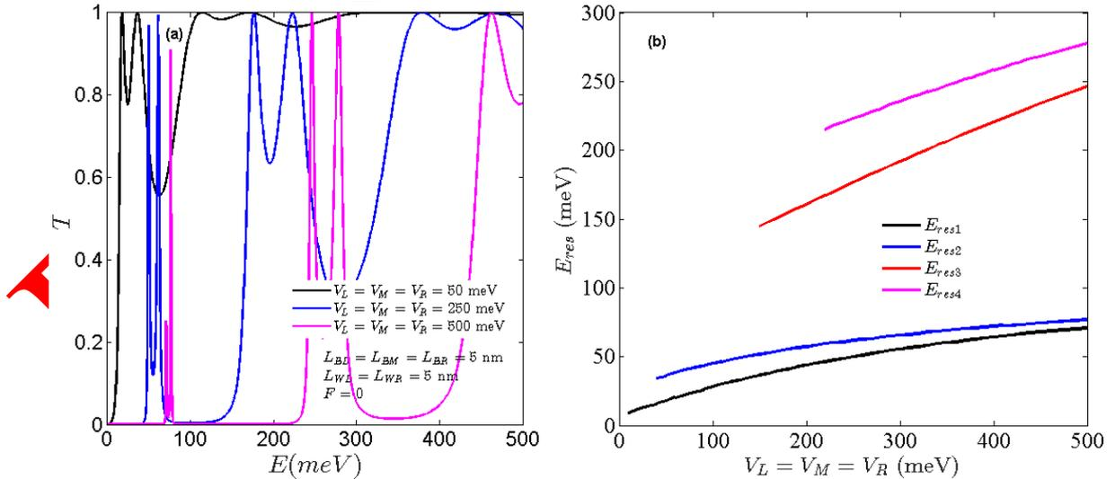
**Figure 2.** (color online) **a)** Graph of the variation of the transmission coefficient with the incident electron energy. Barrier heights vary symmetrically the same  $V_L = V_M = V_R = 50, 250,$  and  $500$  meV. **b)** The graph of resonance energy with barrier heights. System parameters were chosen as  $L_{BL}=L_{BM}=L_{BR}$  5 nm,  $L_{WL} = L_{WR} = 5$  nm and  $F = 0.0$
