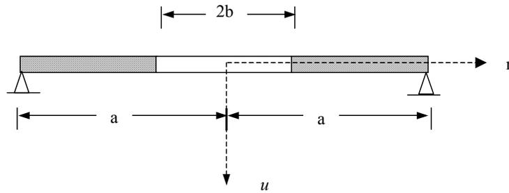
Figure 15. Simply supported annular plates
