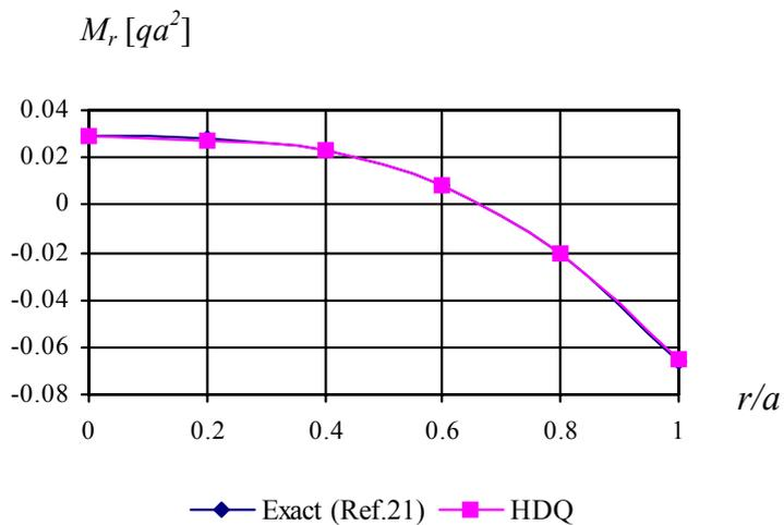
Figure 3. Bending moment in radial direction for clamped edge (CASE 3;  $\nu = 0.3$ )
