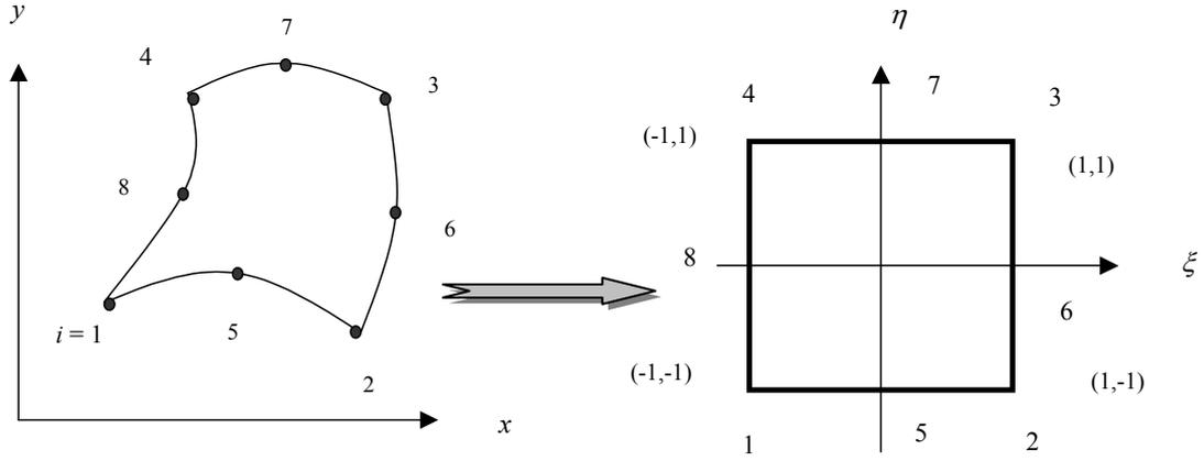
Figure 13(a). Curvilinear quadrilateral domain, (b) standard square domain
