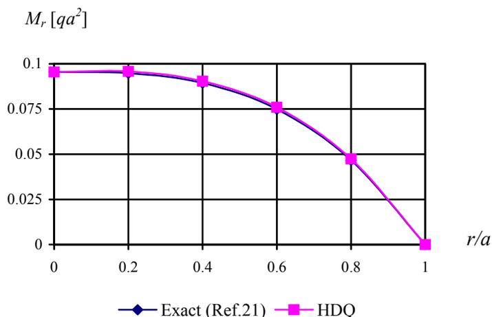
Figure 6. Bending moment in radial direction for simply supported edge (CASE 4;  $\nu = 0.3$ )
