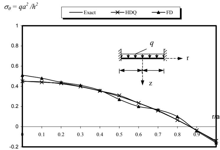
Figure 9. Stress value in tangential direction for clamped plate ( $\nu = 0.2$ )
