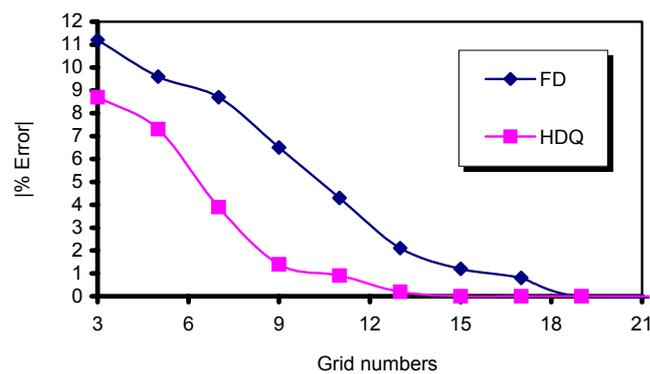
Fig. 12. Percentage error with grid numbers for uniformly loaded simply supported plates (CASE-6;  $\nu = 0.2$ )
