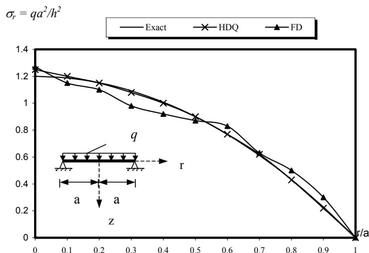
Figure 7. Stress value in radial direction for simply supported plate ( $\nu = 0.2$ )
