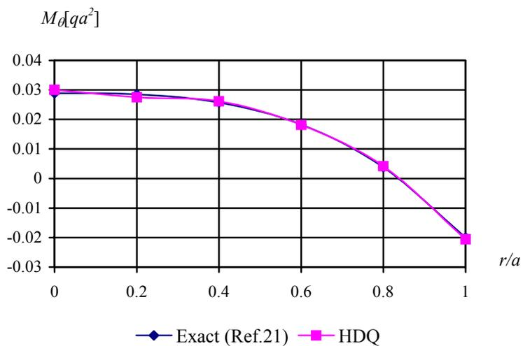
Figure 4. Bending moment in tangential direction for clamped edge (CASE 3;  $\nu = 0.3$ )
