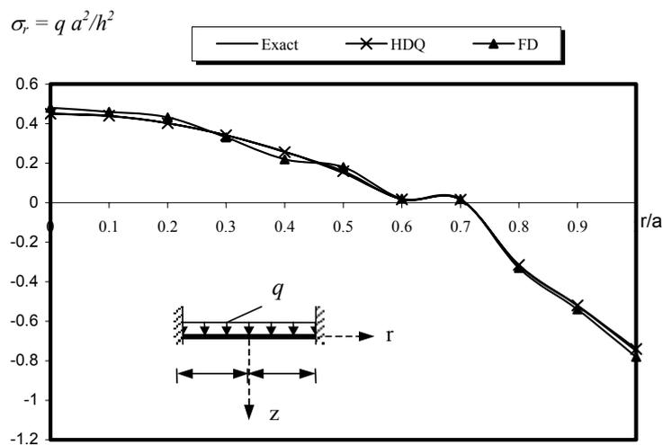
Figure 8. Stress value in radial direction for clamped plate ( $\nu = 0.2$ )
