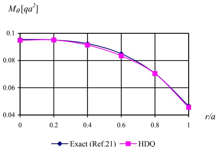
Figure 5. Bending moment in tangential direction for simply supported edge (CASE 4;  $\nu = 0.3$ )
