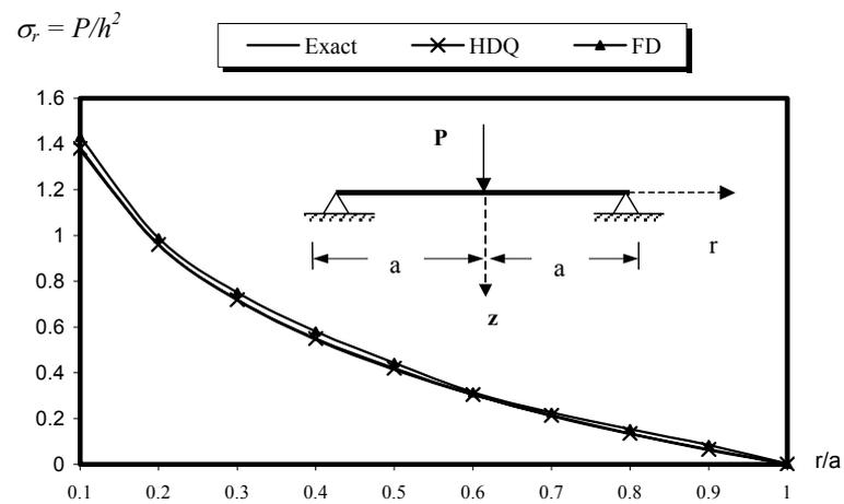
Figure 10. Stress value in radial direction for simply supported plate ( $\nu = 0.25$ )
