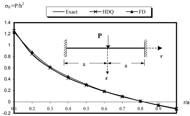
Figure 11. Stress value in tangential direction for clamped plate ( $\nu = 0.25$ )
