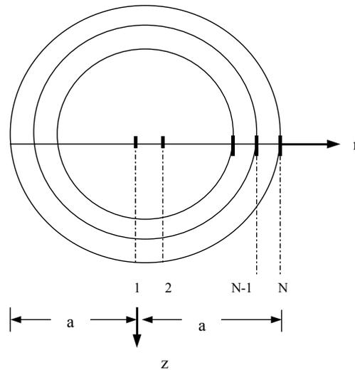
Figure 1. Grid spacing for a thin circular plate
