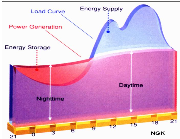
Figure 1. Load leveling cycle [4].
