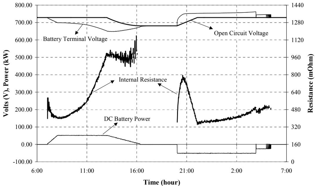
**Figure 8.** The battery total internal resistance, open circuit voltage, dc power, and the terminal voltage of the NAS battery module.
