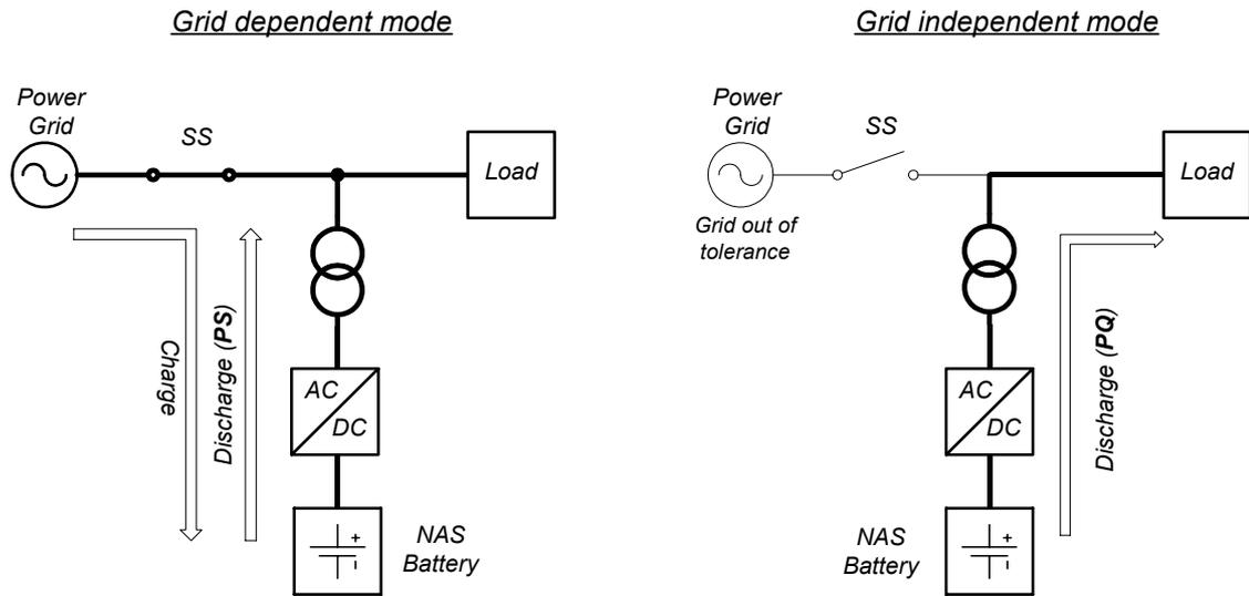
**Figure 4.** Simplified version of the NAS battery system shown in Figure 3 [6].
