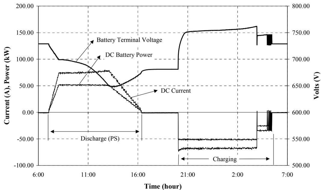
**Figure 6.** The dc power, current, and terminal voltage of the NAS battery module during a daily discharge and charge cycle.
