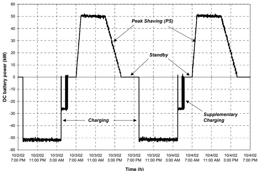
**Figure 5.** The operational pattern of the NAS battery system for one day of testing. The pattern includes peak shaving, charging, supplementary charging, and standbys.
