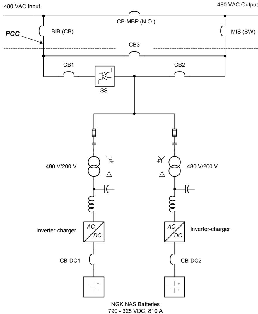
**Figure 3.** One line diagram of the implemented multi-function NAS battery energy storage system.
