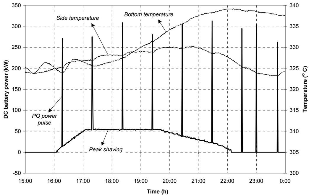
**Figure 9.** Combined operation-PS with 250kW PQ protection for 30 seconds. The upper two waveforms show the base and the side battery module temperatures.
