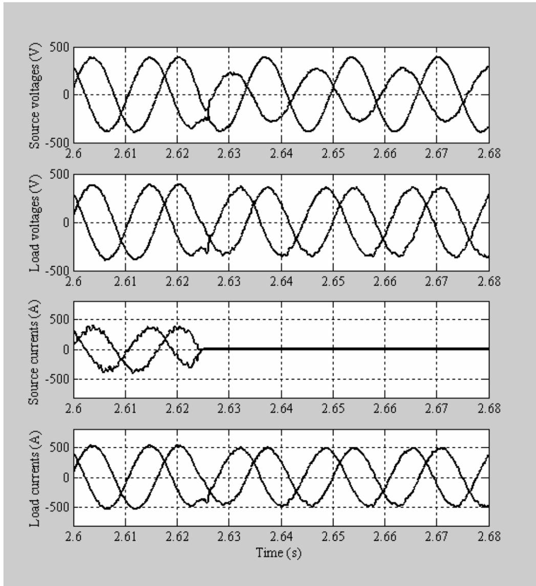
**Figure 10.** The system response to a PQ event test during a peak shaving cycle. The top trace shows only the two phases (*a*, *b*) of the power system, the second trace is the load voltages, the third trace is the source currents and the bottom trace is the load currents.
