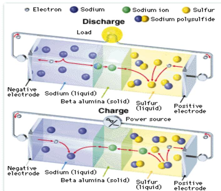
Figure 2. A simple diagram that shows the electrochemical reactions inside a NAS battery [4].
