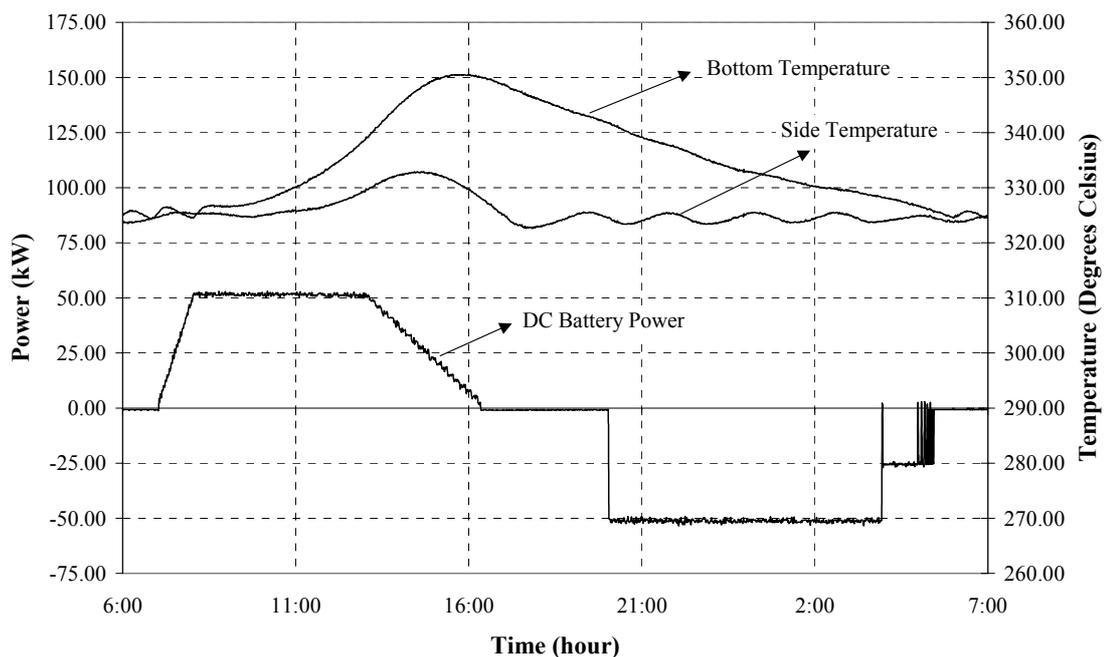
**Figure 7.** The dc power, side and bottom temperatures of the NAS battery module.
