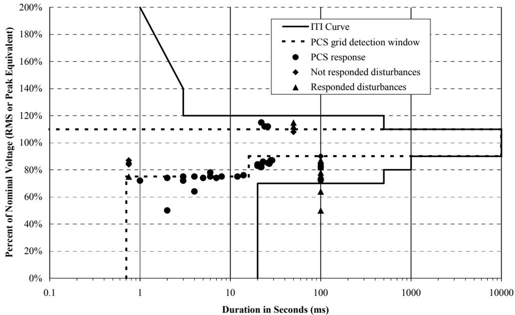
**Figure 11.** ITIC compliance test results of the NAS Battery system.
