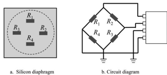
**Figure 1.** Schematic of Manifold Absolute Pressure Sensor [4]
