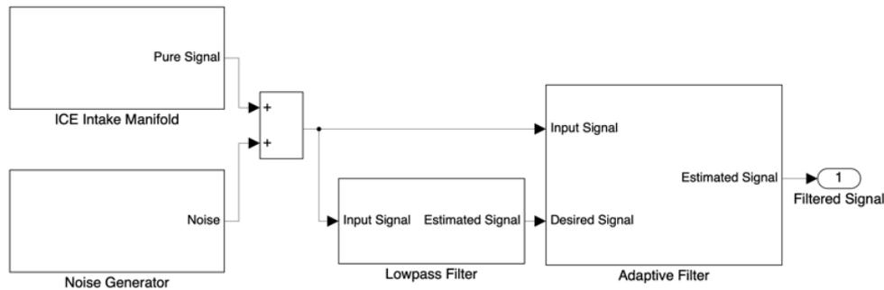
**Figure 4.** Signal Processing Schematic of Adaptive Filtering
