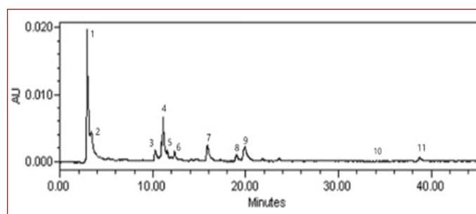
**Figure 1.** The HPLC chromatogram (360nm) of the phenolic substances in the Zj fruit extract. Peak identification; 1 Gallic acid; 2 protocatechuic acid; 3 syringic acid; 4 catechin; 5 epigallocatechin; 6 p-coumaric acid; 7 ferulic acid; 8 ellagic acid; 9 rutin; 10 t-cinnamic acid; 11 kaempferol
