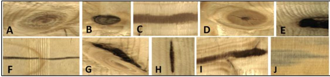
**Figure 1.** Images of 10 common defect types of the dataset: (A) Live Knot, (B) Dead Knot, (C) Quartzity, (D) Knot with crack, (E) Knot missing, (F) Crack, (G) Overgrown, (H) Resin, (I) Marrow (J) Blue stain.
