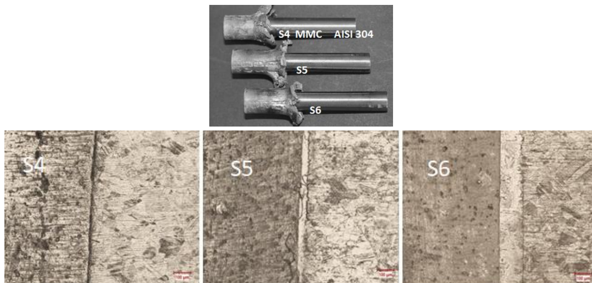
Figure 2. The microstructure in the welding zone of the friction welds by using 1500 rpm rotation speed.
