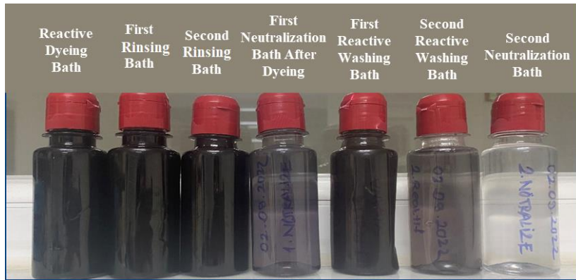
Figure 6. Conventional dyeing baths wastewater
