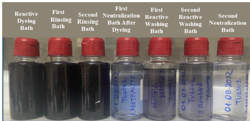
Figure 7. Salt-free dyeing baths wastewater
