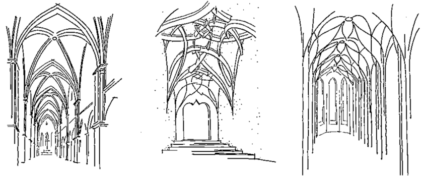
Figure 3: Different rib vault structures (Siegel, 1962).
