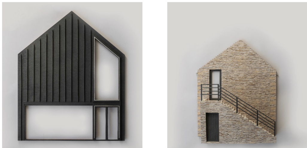
Figure 12-13. 1:20 Models comparing Pier Arts Centre's Tradition and Contemporary Gable Ends
