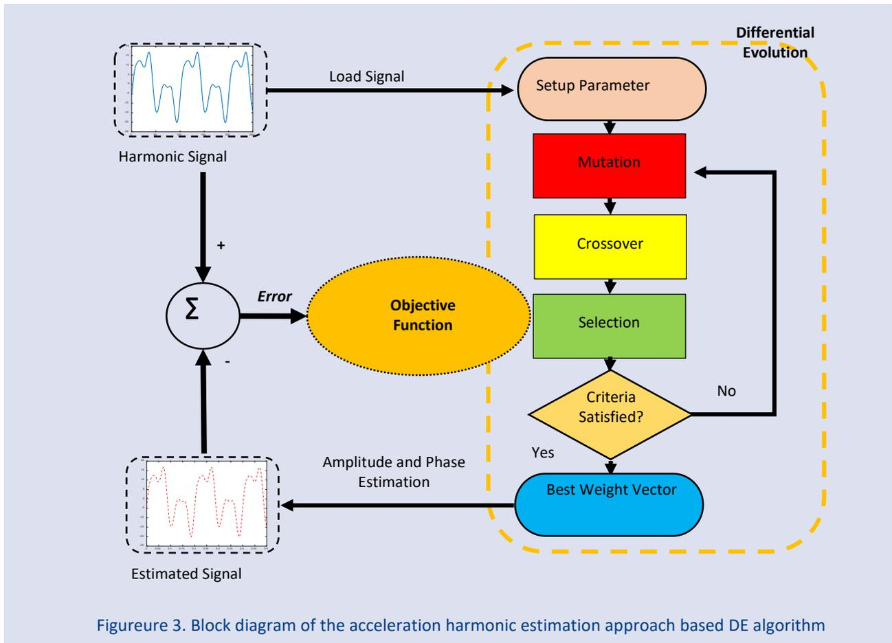
Figure 3. Block diagram of the acceleration harmonic estimation approach based DE algorithm
