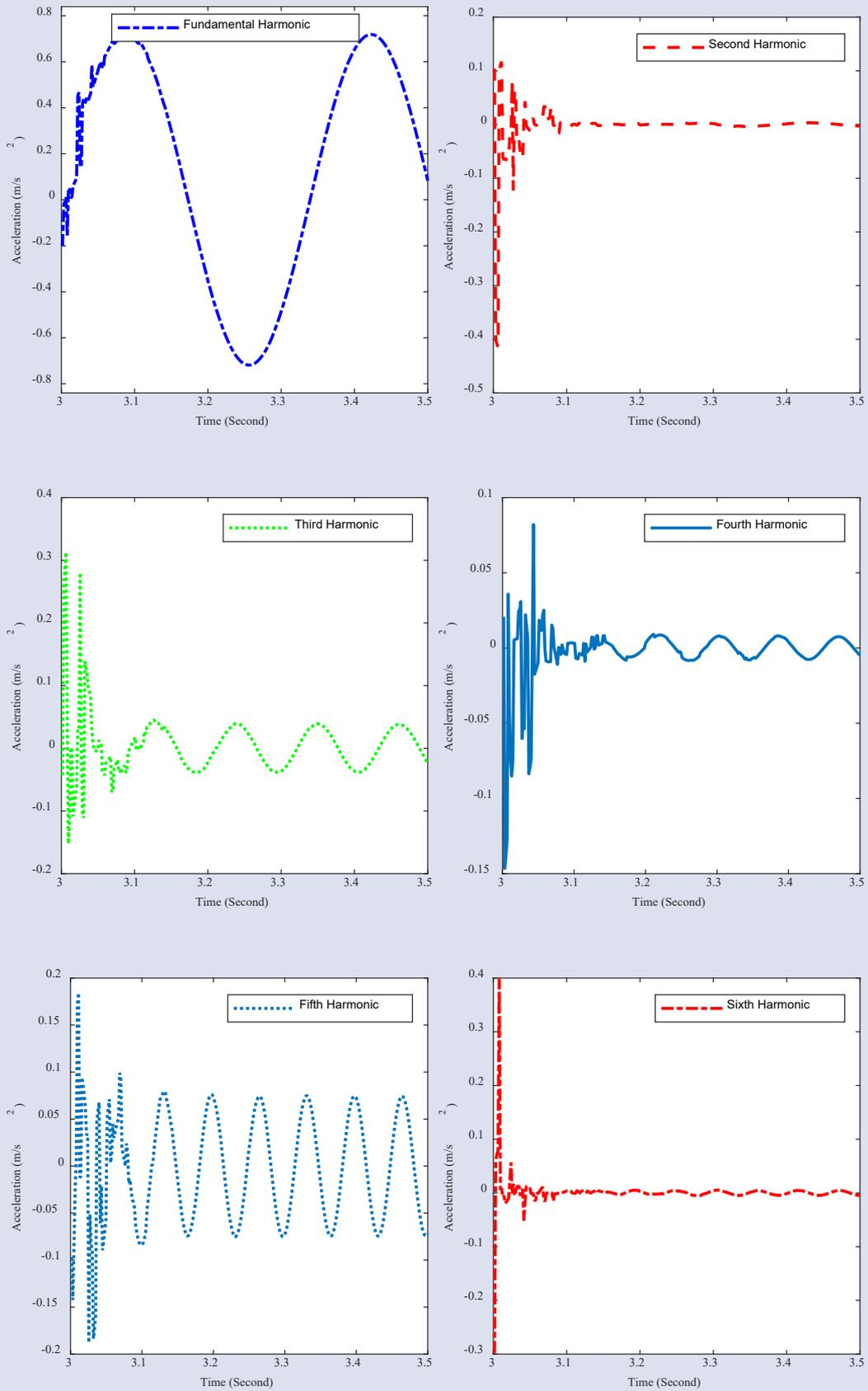
Figure 11. Harmonic waveforms by generating estimated amplitude and phase values
