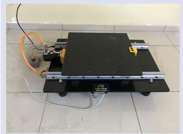
Figure. 1. Servo Electro-Mechanical Shaking Table
