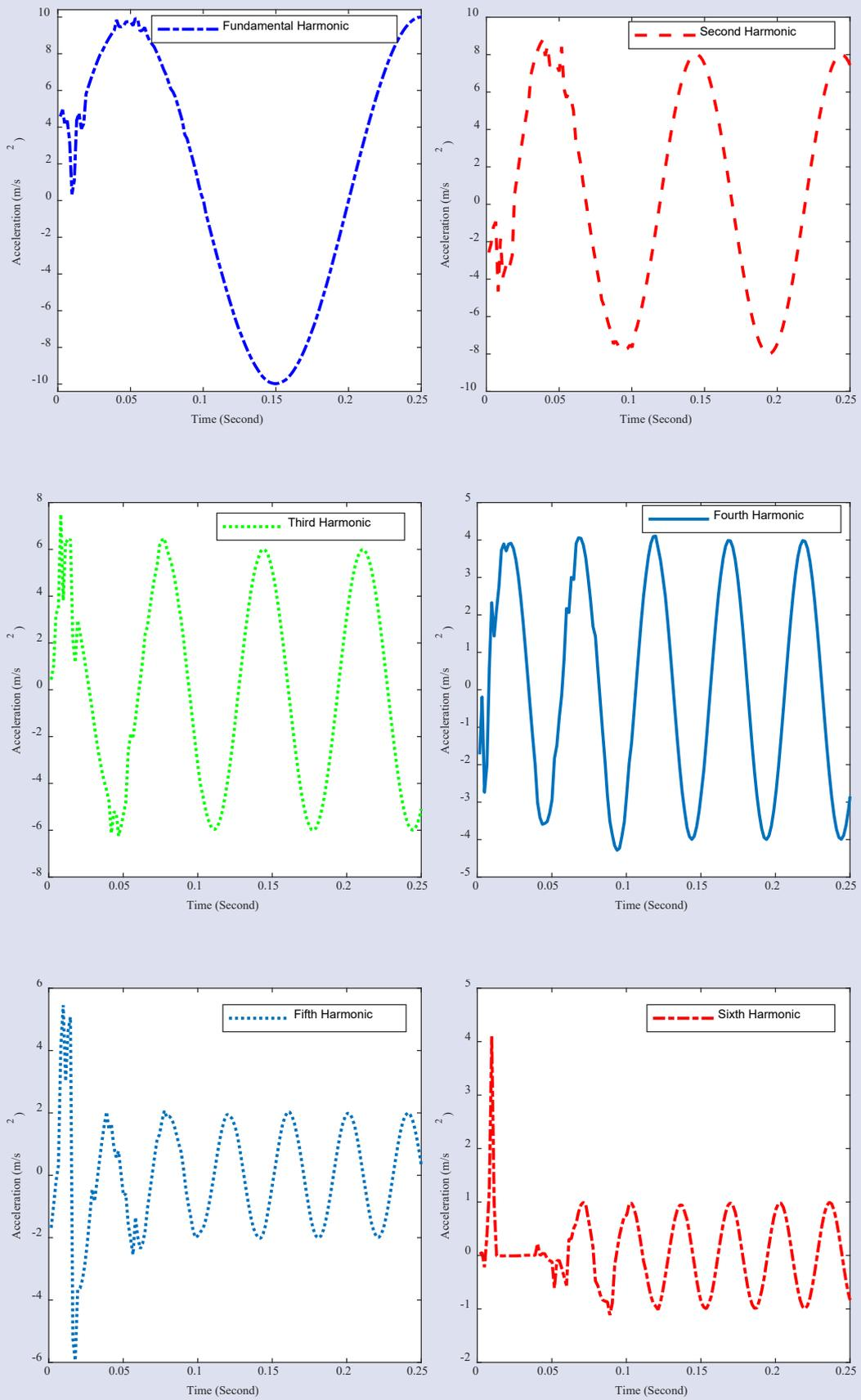
Figure 7. Harmonic waveforms by generating estimated amplitude and phase values
