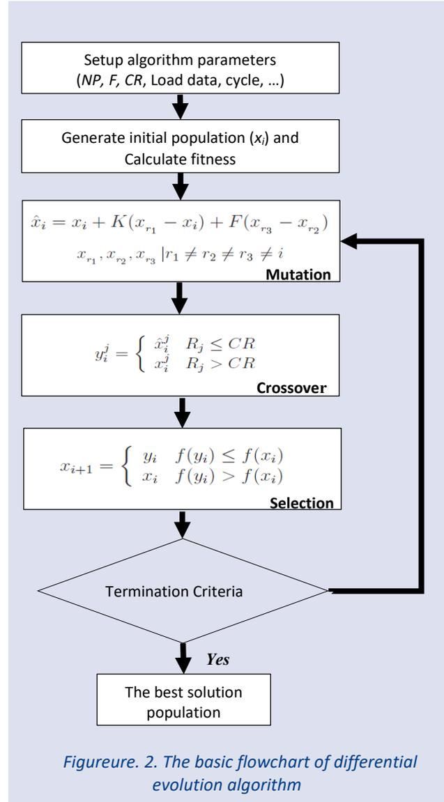
Figure. 2. The basic flowchart of differential evolution algorithm
