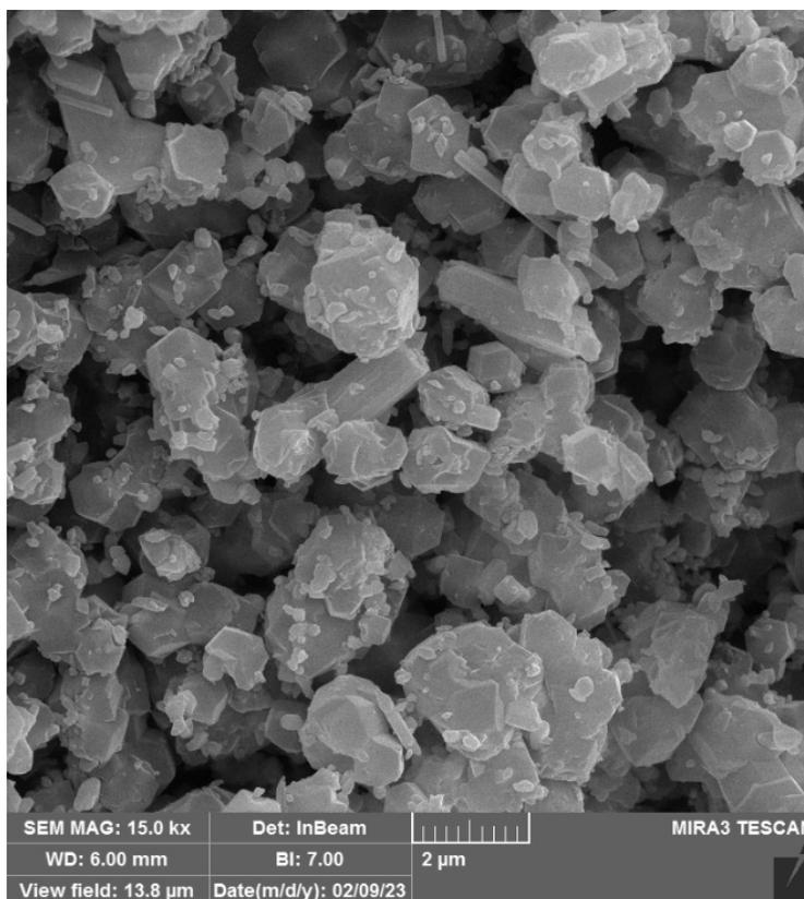
Figure 1. FESEM image of (ZnO@ZIF-8) composite
