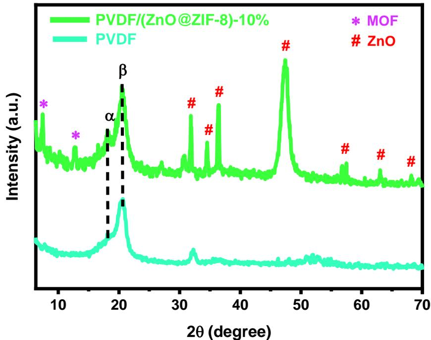
Figure 4. X-ray diffraction of PVDF and PVDF/(ZnO@ZIF-8)-10% nanofibers
