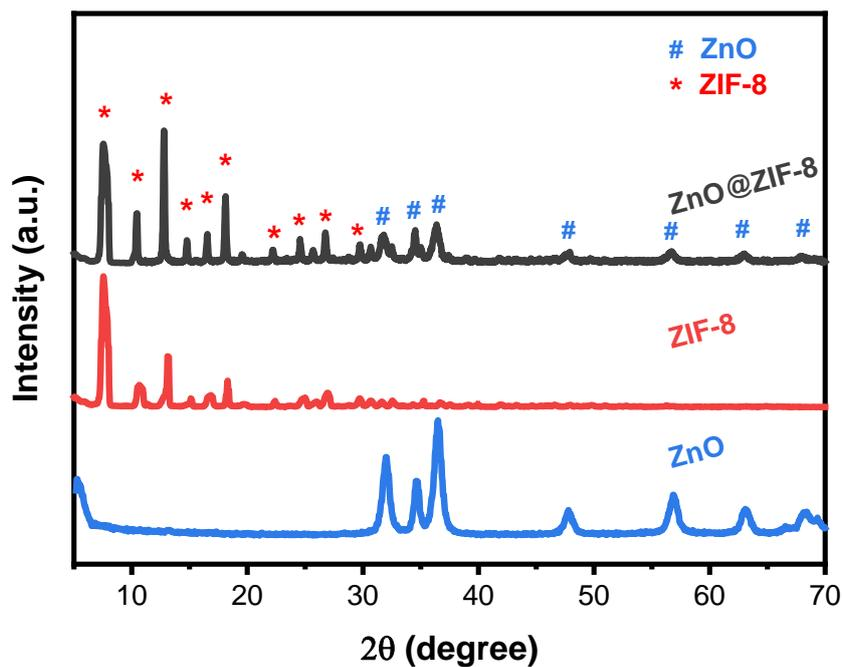
Figure 2. X-ray diffraction pattern of ZnO, ZIF-8 and (ZnO@ZIF-8) powders
