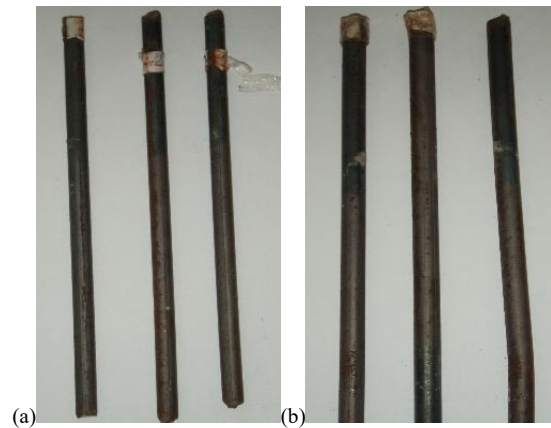
Fig. 15 Corrosion activity of reinforcing bars (a) M1A and (b) M2A
