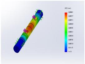
Figure 15. Representation of Displacement of Transmission Shaft
