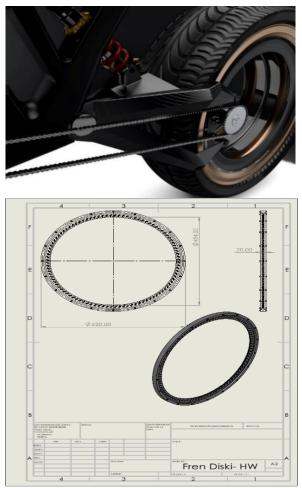
Figure 16. Technical Drawing of Brake Disc
