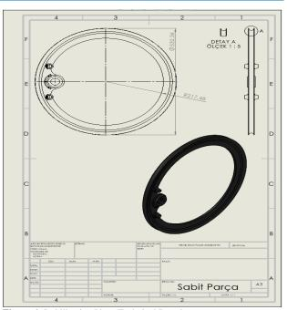
Figure 6. Stabilization Piece Technical Drawing
