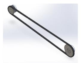
Figure 12. Assembly of Sprocket Gear Transmission
