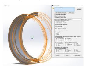
Figure 1. Mass measurement results of hubless rim design
