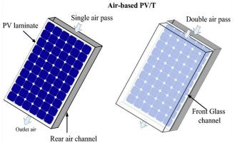
Figure 2 Air based PV/T (single and double) [15]
