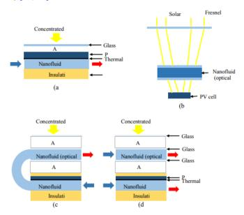
Figure 6 Schematic diagrams of PVT system with nanofluid [33]
