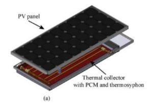
Figure 5 Cooling with PCM [27]
