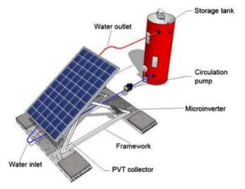
Figure 3 Water cooling [20]
