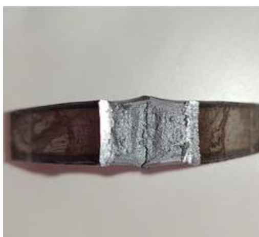
Fig. 3 Photograph of the sample after impact testing
