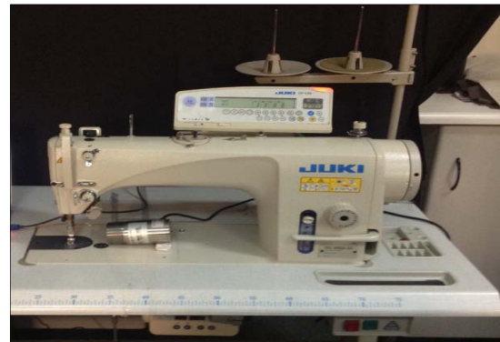
Figure 5. Needle temperature measurement setup
