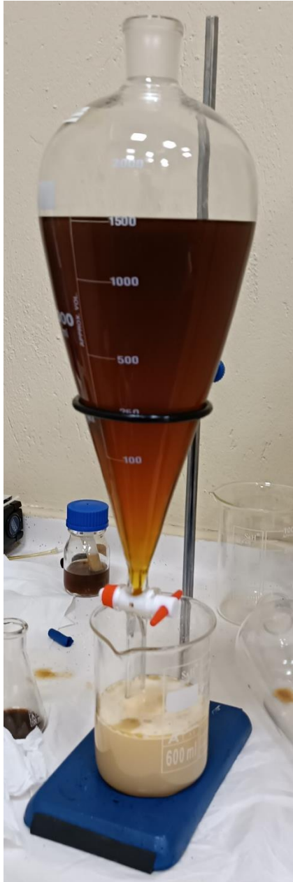
Fig. 2. Separation of washing water with a separating funnel.
