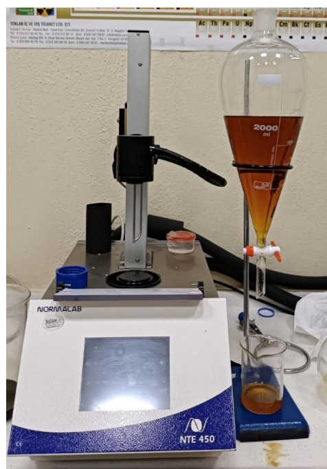
Fig. 1. Separation of glycerol with a separatory funnel.
