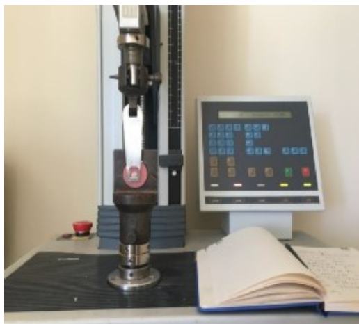
Figure 4: Shear connection strength test
