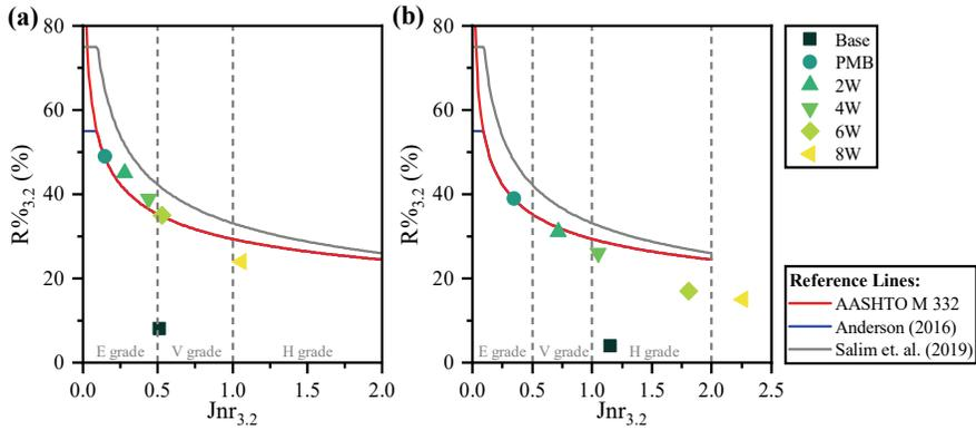
Figure 6 - Comparison of  $Jnr_{3,2}$  and  $R\%_{3,2}$  values of bitumen samples with reference curves for polymer network detection at different temperatures: (a) 58°C and (b) 64°C.
