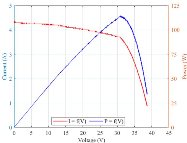
Fig. 7. Experimental graph of I-V and P-V specifications.
