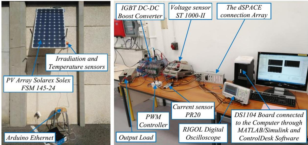
Fig. 6. The hardware configuration used in the experiment.
