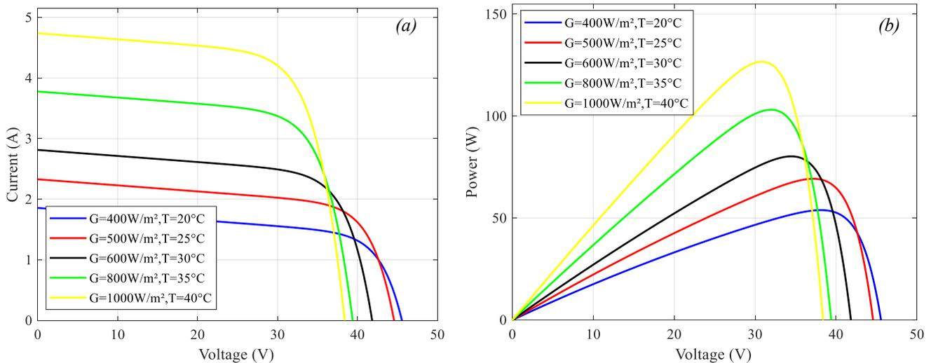
Fig. 3. Effect of temperature and irradiance occurring simultaneously, (a)  $I-V$  and (b)  $P-V$  characteristic.
