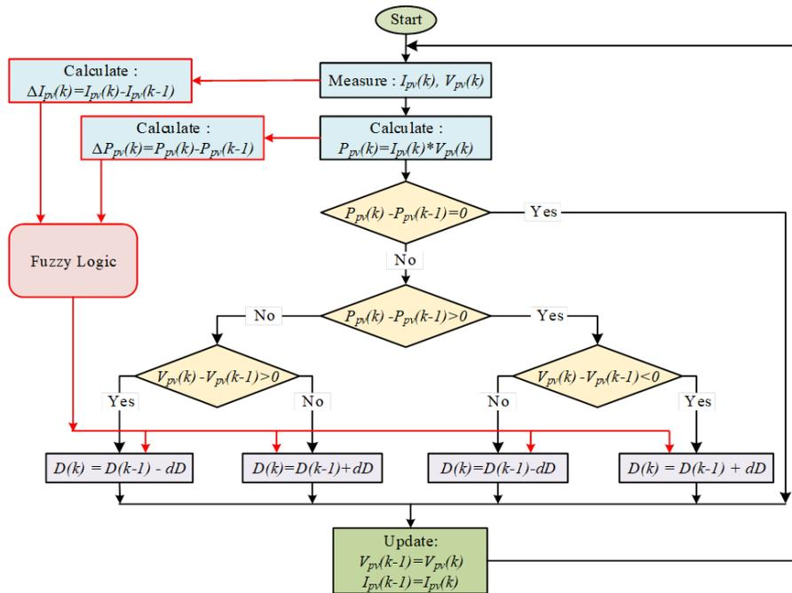
Fig. 5. Flowchart of perturbation and observation strategy improved by FL with a variable step.
