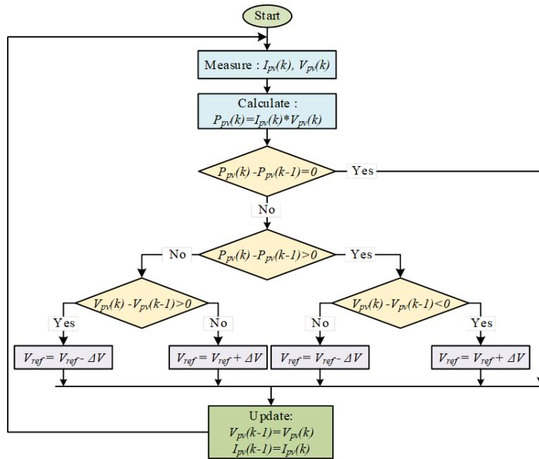
Fig. 4. Conventional P&O algorithm flowchart.
