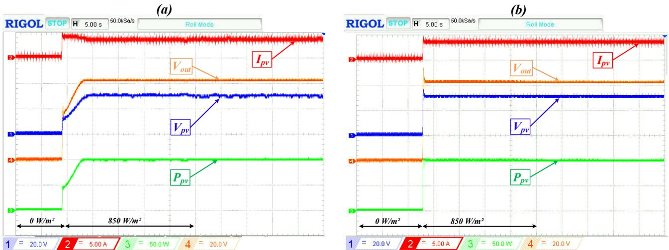
Fig. 8. Results from experiments, (a) classic P&O and (b) improved PandO approach by FLC.
