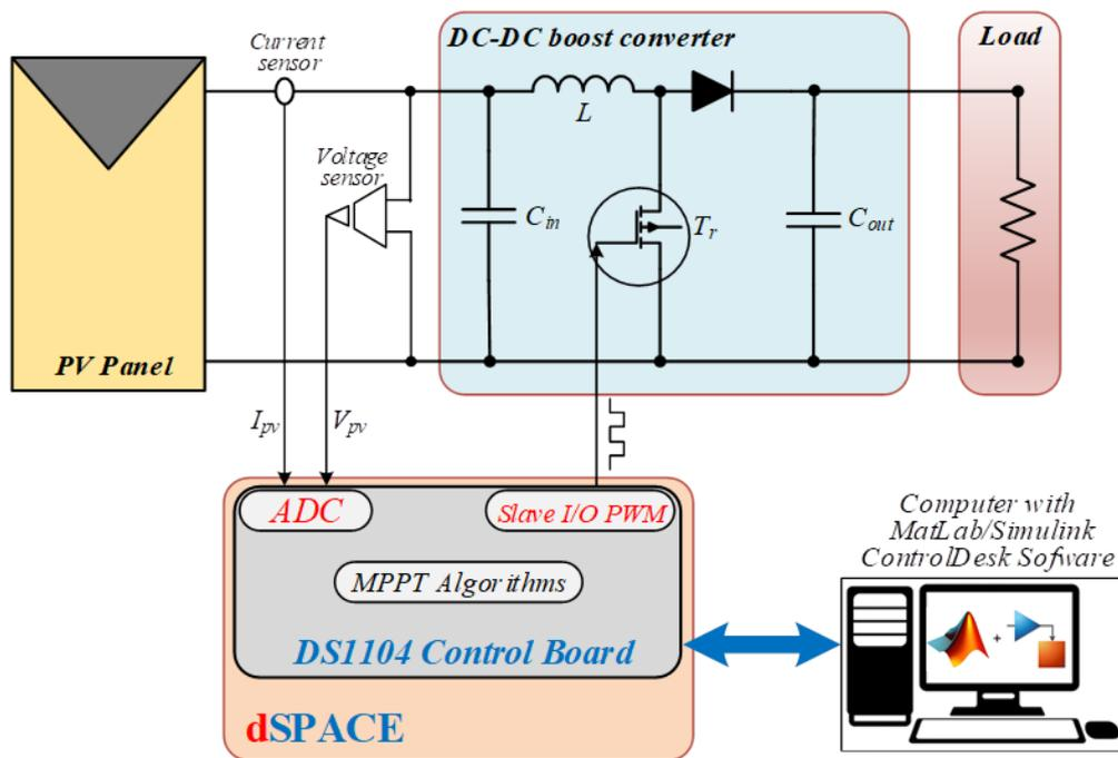
Fig. 1. Schematic diagram of the proposed solar power system.
