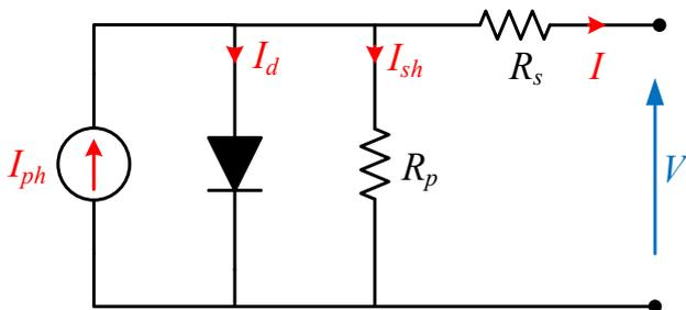
Fig. 2. Single diode solar cells electrical layout.
