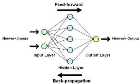
Figure 2. Artificial Neural Network Structure.
