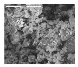
Figure 2: SEM photographs of egg shell (calcite).
