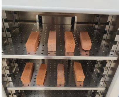
Figure 3. Drying the samples in an furnace
