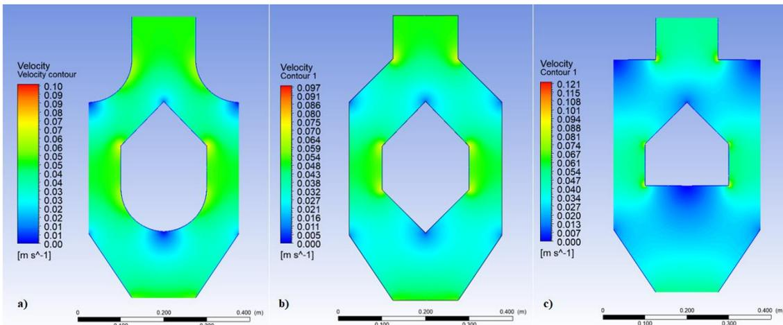
Figure 7. Velocity contours a) Circular b) Angular c) Straight
