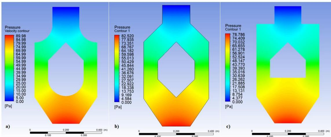
Figure 8. Pressure contours a) Circular b) Angular c) Straight
