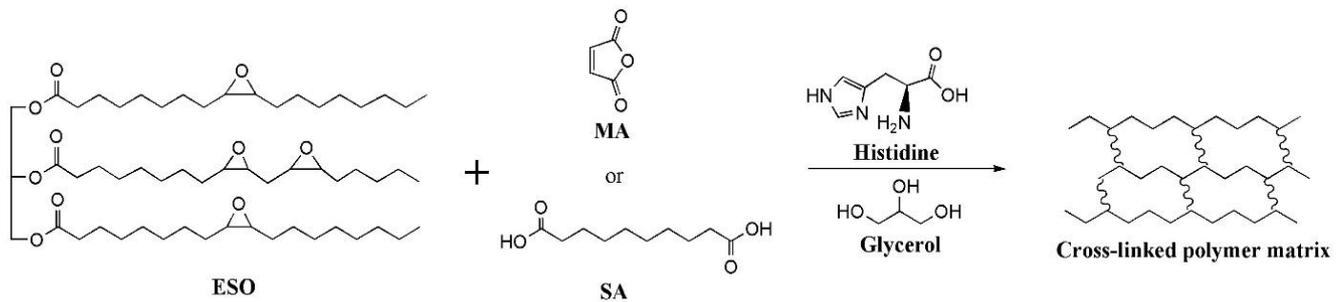
**Figure 1.** Schematic presentation of polymer matrix preparation with ESO
