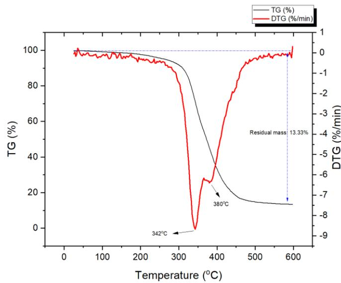
**Figure 7.** TGA-DTG curves of 4 plies hemp fabric reinforced MAESO composite material
