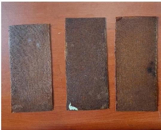
**Figure 5.** Hemp fiber reinforced composite samples
