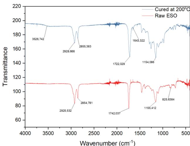
**Figure 9.** FTIR spectra of raw ESO and cured composite sample
