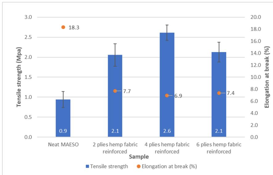
**Figure 3.** Tensile strength and elongation at break values of hemp fiber reinforced composites
