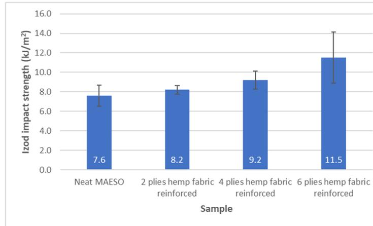
**Figure 6.** Izod impact test results of the hemp-MAESO composites
