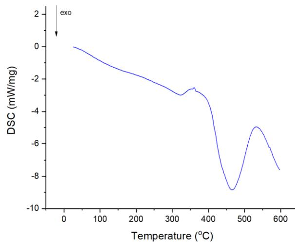
**Figure 8.** DSC curve of 4 plies hemp fabric reinforced MAESO composite material
