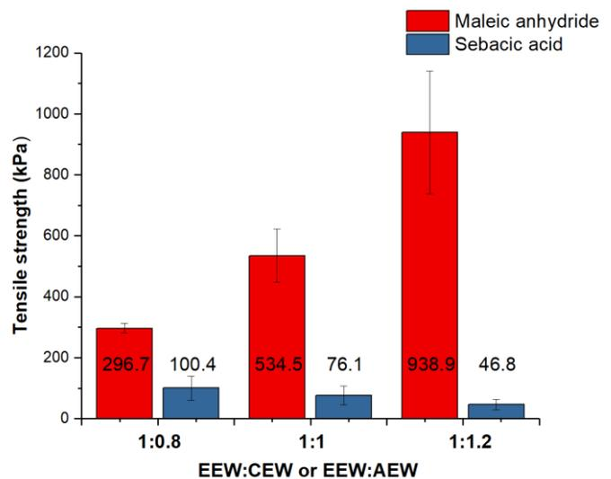
**Figure 2.** Tensile strength values of neat polymer matrices produced with MA or SA hardeners
