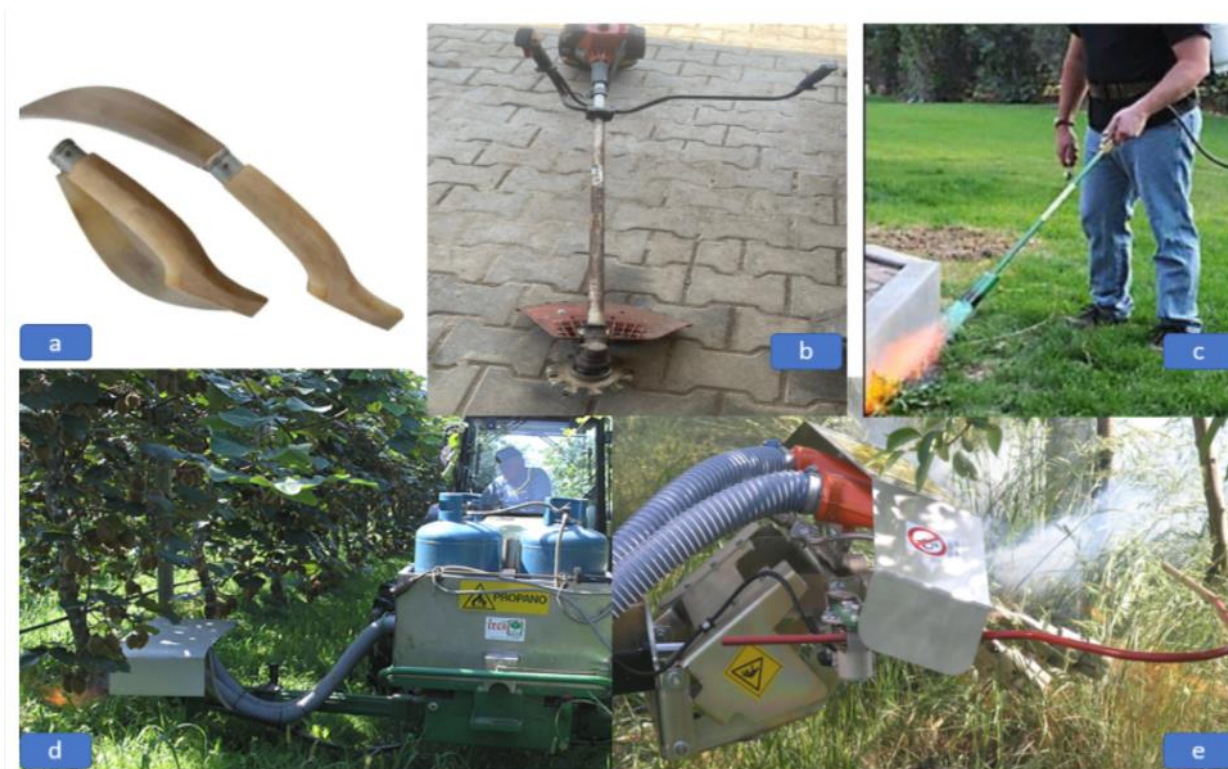
Figure 2. Tools and machines used in the control of the suckers, a. Hazelnut knife (Anonymous 2023a), b. Sucker mower, c. Back-mounted flamethrower (Anonymous 2023b), d. Tractor-pulled flamethrower (Anonymous 2023c), e. Steam machine (Anonymous 2023d).
