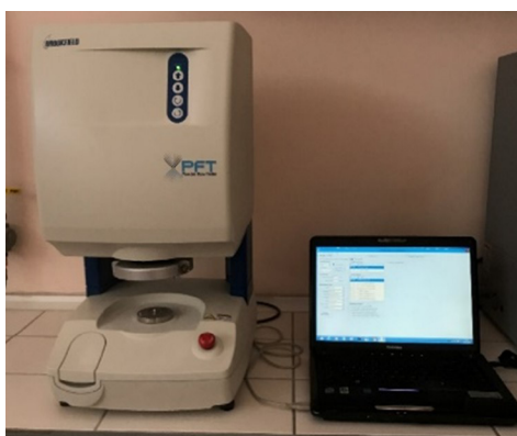
Figure 2. Powder flow tester
