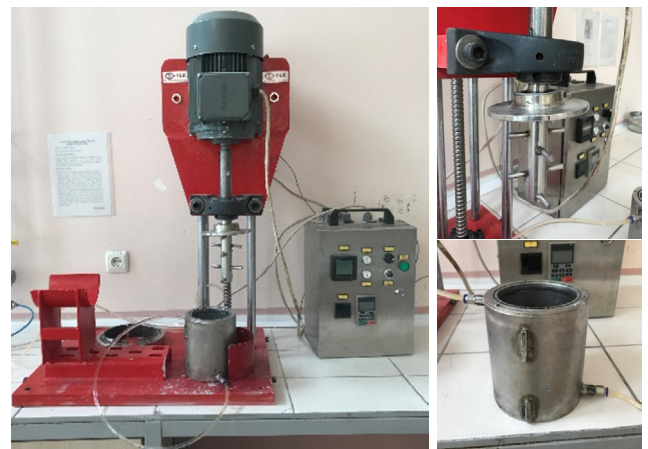
Figure 1. Vertical batch-type laboratory stirred ball mill, pin-type stirrer and grinding tank
