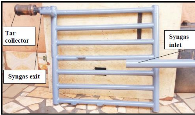
Fig. 5: Fabricated syngas cooler
