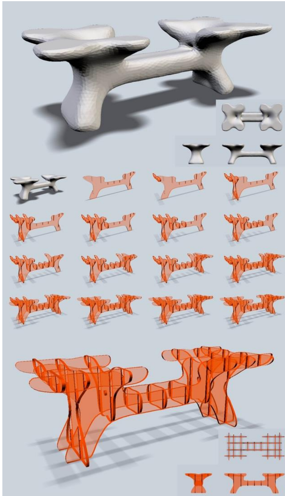
Figure 8. Waffle structure. (top) Volume reduction resulting from optimization; (middle) Installation sequences; (bottom) Final slices.
