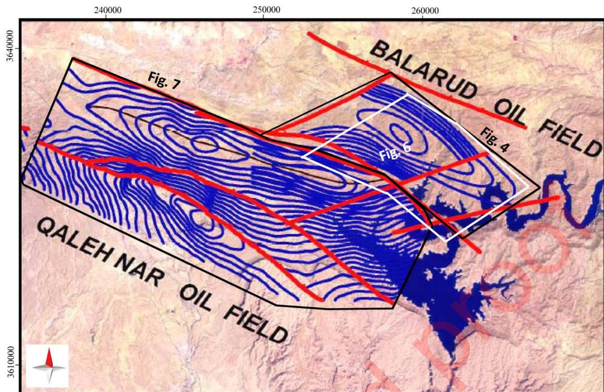
**Fig. 2.** UGC map of the studied anticlines on the satellite image. The location of this Figure is shown in Fig. 1B.
