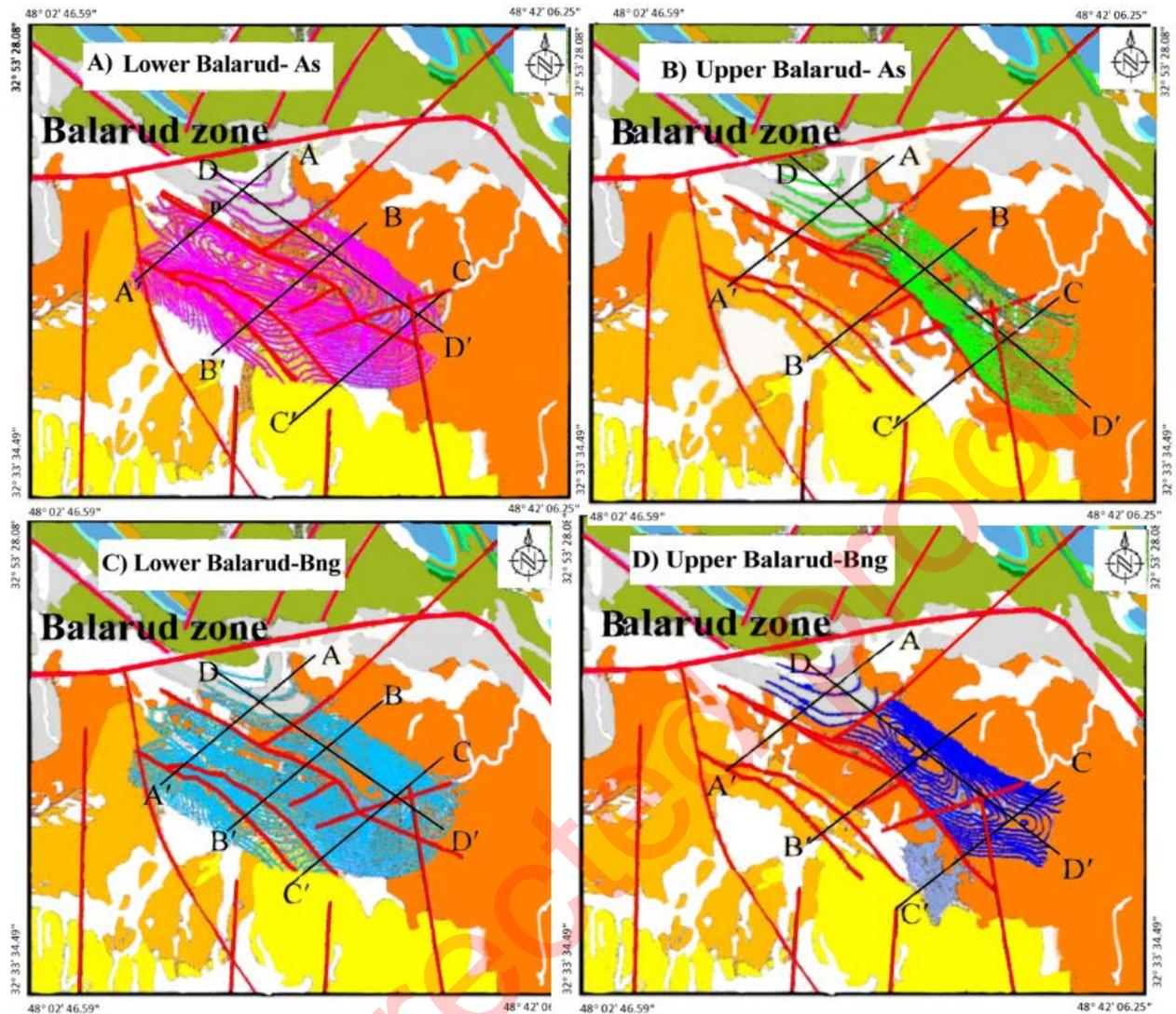
**Fig. 11.** Geological map (with a scale of 1:100000) of the study area (Legend in Fig. 1B) and location of the structural sections (AA'-DD'). Contours are the UGC map (As and Bng) for UBR, LBR and QN anticlines and indicate the location of these anticlines. Red lines show faults.
