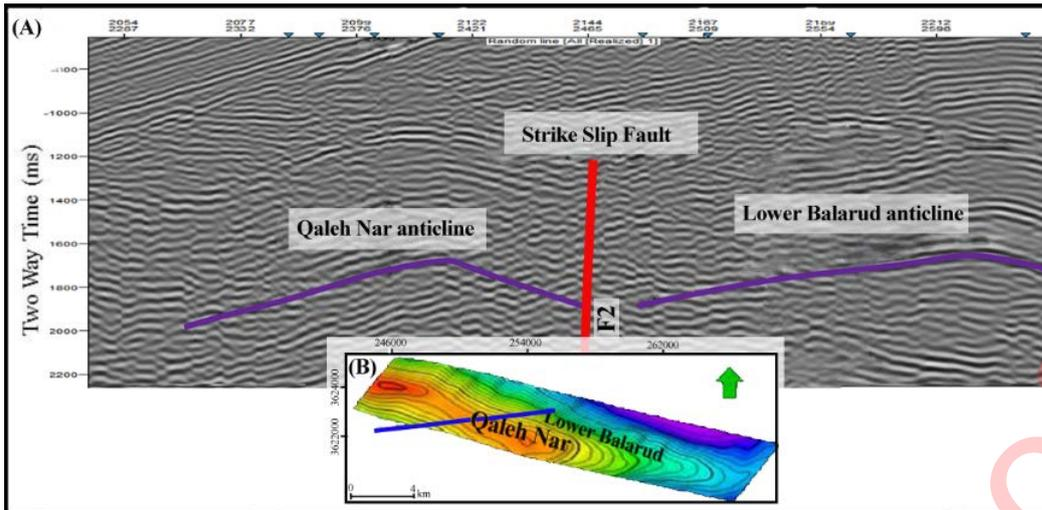
**Fig. 6.** Bangestan horizon (purple lines) in the *LBR* and *QN* anticlines on the (A) seismic profile and (B) UGC map. The red line indicates F2. The blue line shows the location of the seismic profile on the UGC map.
