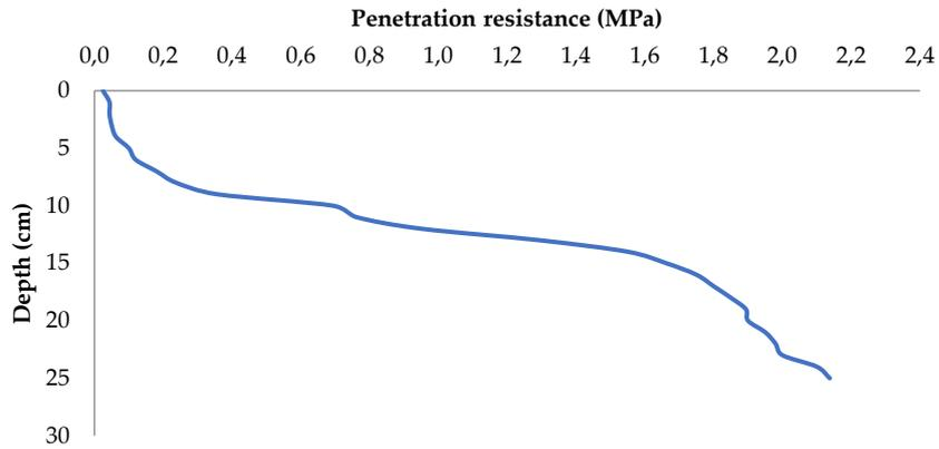
Figure 5. Penetration resistance curve of seed bed
