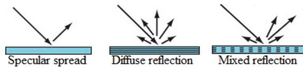
Figure 8. Reflecting light by surface type.
