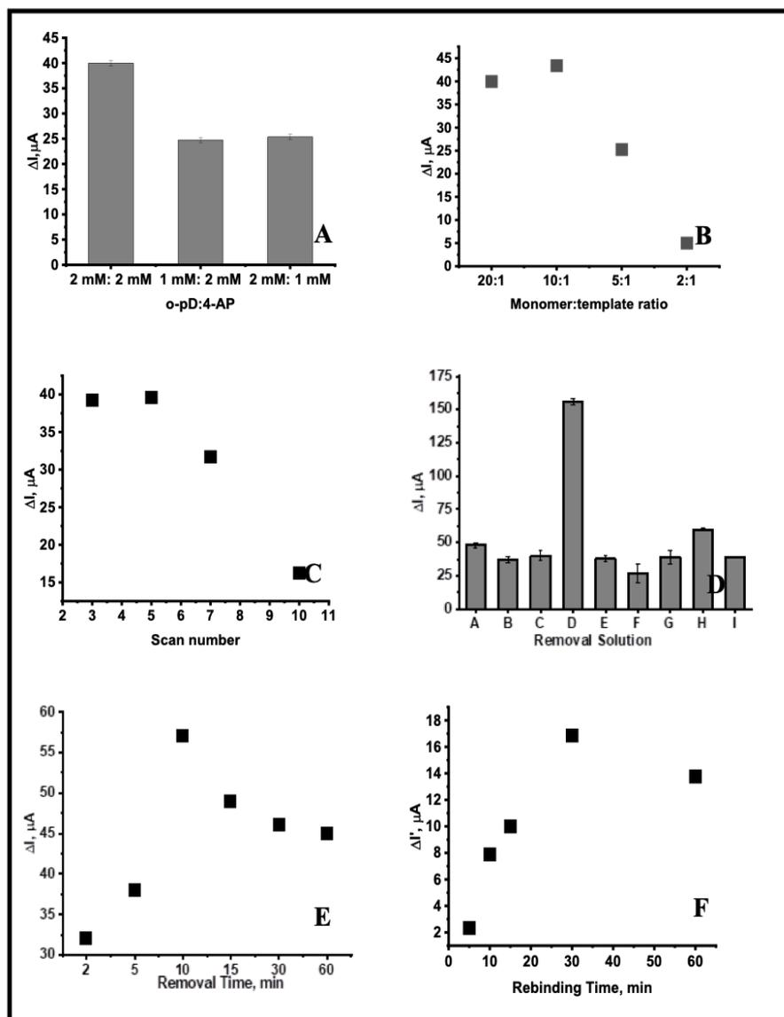
**Figure 3.** The optimization studies of o-pD:4-AP monomer ratio(A), monomer: template ratio(B), number of electropolymerization scan(C), removal solution(D), removal time(E) and rebinding time(F) for development of MIP(PERA)/GCE
