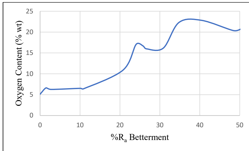
Figure 21. The relationship between %R a betterment rate and the amount of Oxygen contained
