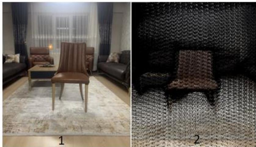
**Figure 12.** A sample point cloud data taken from the experimental environment in real time with the iPhone built-in LIDAR sensor
