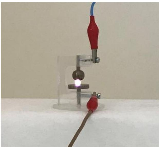
Figure 11. Corona discharge image at high frequencies in the electrode system of Sphere-Plane
