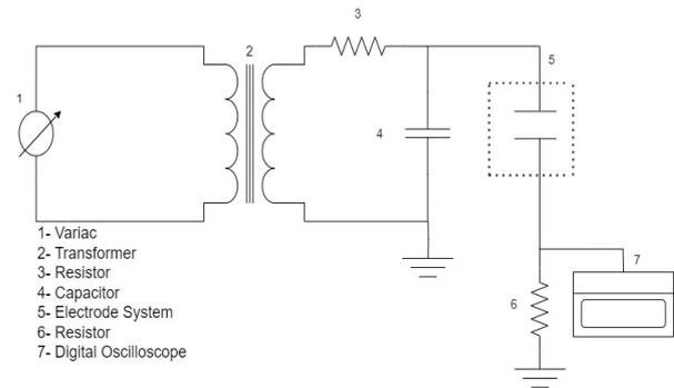
Figure 3. Circuit diagram of the experimental setup
