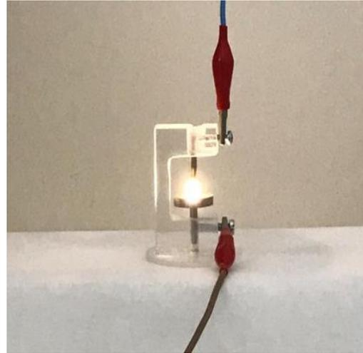
Figure 5. Corona discharge image at low frequencies in the electrode system of Needle-Plane
