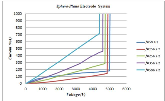
Figure 12. Voltage-Current change graph for the electrode system of Sphere-Plane, obtained at various supply voltage frequencies.
