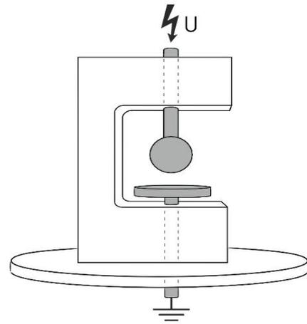
Figure 2. Sphere-Plane electrode system image
