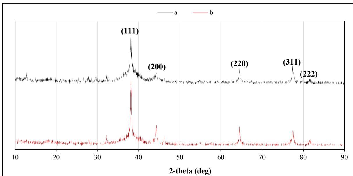
**Figure 4.** XRD patterns of the nanomaterials synthesized at the proportions of a and b
