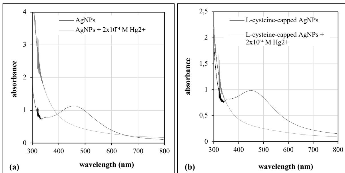
**Figure 6.** The colorimetric Hg<sup>2+</sup> detection performance of (a) AgNPs and (b) L-cysteine-capped AgNPs
