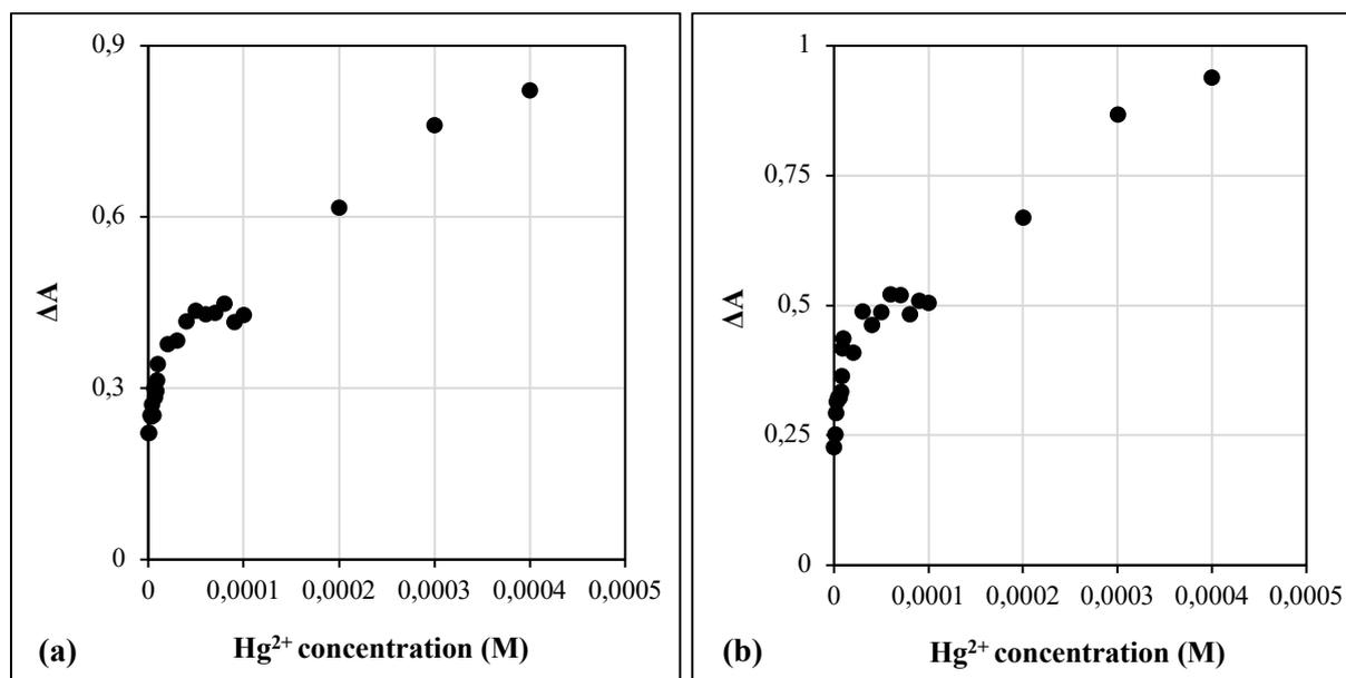
**Figure 8.** The changes of absorbance differences with Hg<sup>2+</sup> concentrations for (a) AgNPs and (b) L-cysteine-capped AgNPs
