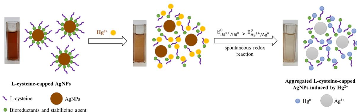
**Figure 7.** The proposed detection mechanism of Hg<sup>2+</sup> with L-cysteine-capped AgNPs
