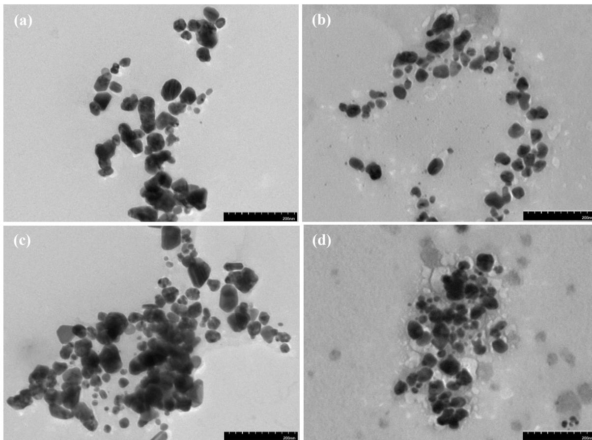
**Figure 5.** TEM images of the nanomaterials synthesized at the proportions of a and b, (c) and (d) TEM images of the nanomaterials synthesized at the proportions of a and b after Hg<sup>2+</sup> detection, respectively
