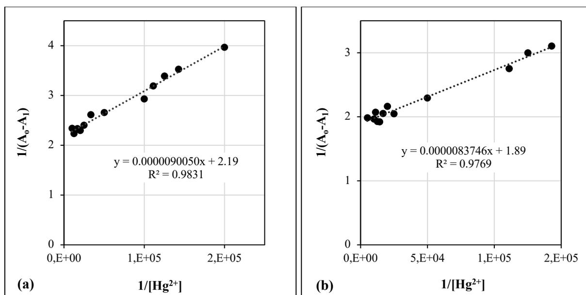
**Figure 9.** The linear relationship based on the Benesi–Hildebrand Equation for the formation of (a) Hg<sup>2+</sup>–AgNPs complex and (b) Hg<sup>2+</sup>–L-cysteine-capped AgNPs complex
