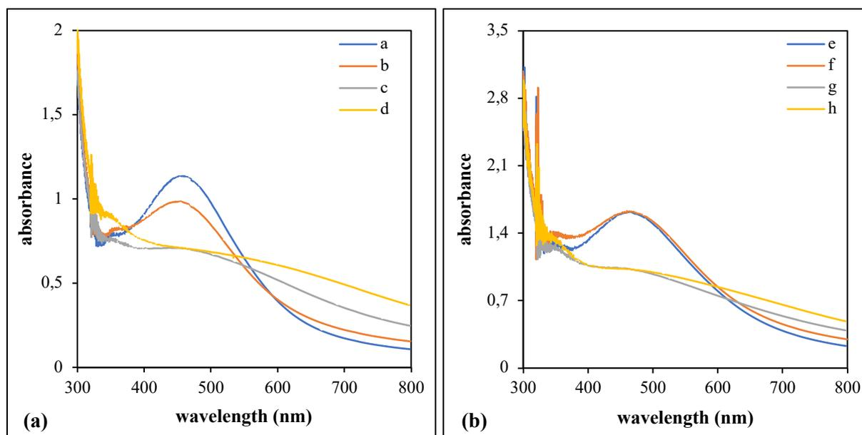
**Figure 2.** The UV-vis spectra of the synthesized nanomaterials in different proportions of the components (a) nanomaterial code: a-d, (b) nanomaterial code: e-h
