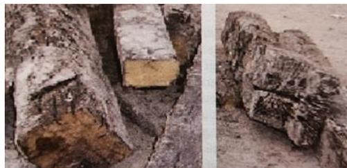
**Figure 2.** Cross sections of water-logged hardwood, Yenikapı Wrecks, İstanbul [9].
