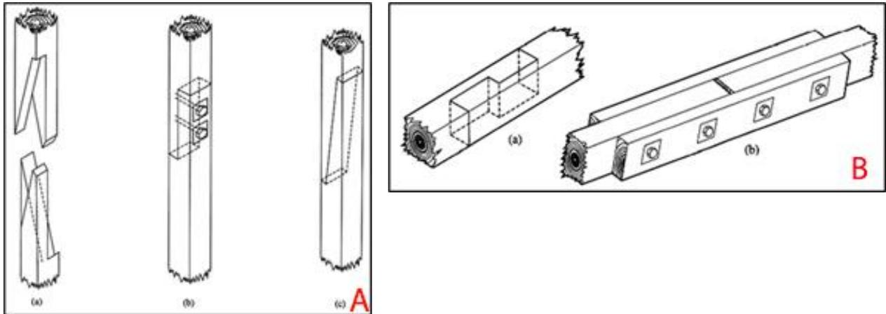
**Figure 6.** (A) Splices for replacement compression timbers: (a) 'scissor-scarf'; (b) simple, bolted scarf; (c) 'self-locking scarf' [24].
