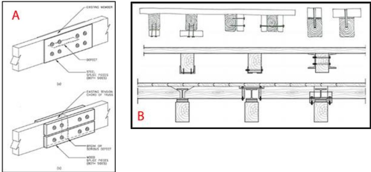
**Figure 13.** (A) Reinforcing damaged members by adding side pieces: (a) using a steel splice plate to reinforce a beam with a serious defect; (b) using wood side pieces to repair the broken bottom chord of a truss [22]. (B) Examples of reinforcement techniques of timber floor beams [30].
