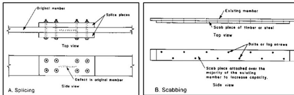
**Figure 8.** Splicing and scabbing methods of member augmentation [27].
