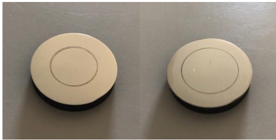
Figure 21. Wear marks on the D2 steel sample after testing with the (a): manufactured tribometer, (b): CSM tribometer
