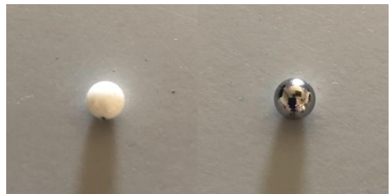
Figure 22. (a): Alumina ( Al_2O_3 ), (b): 100Cr6 steel 6mm balls
