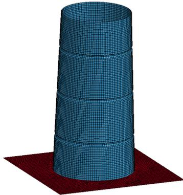
Fig. 4. Finite element mesh of the corrugated crash box
