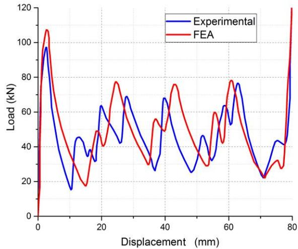
Fig. 5. Experimental and simulation load-displacement curves of crash boxes
