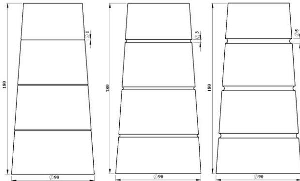
Fig. 2. The geometry of the thin walled tube (with corrugated) having circular cross-section.
