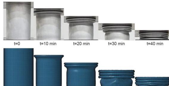
Fig. 6. Deformation of collapse models circular tube from the experimental and numerical results.
