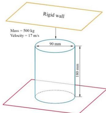
Fig. 3. The crash box impacted with a rigid wall.
