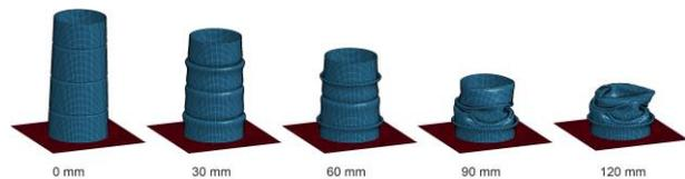
Fig. 9. Deformation photos of CS5.0TA2.0 crash box
