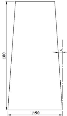
Fig. 1. The geometry of the crash box (without corrugation) having circular cross-section.
