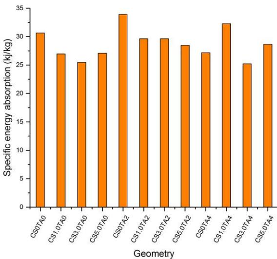
Fig. 8. Specific energy absorption for geometries.
