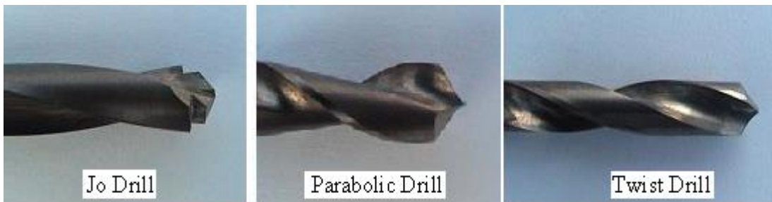
Figure 1. Drill point geometry [34]
