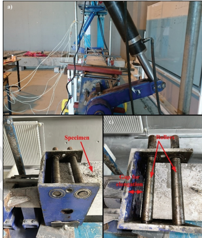
Figure 5 - a) The side view of the test setup, b) Specimen in the headpiece, c) Details of the headpiece of the test setup for elongation
