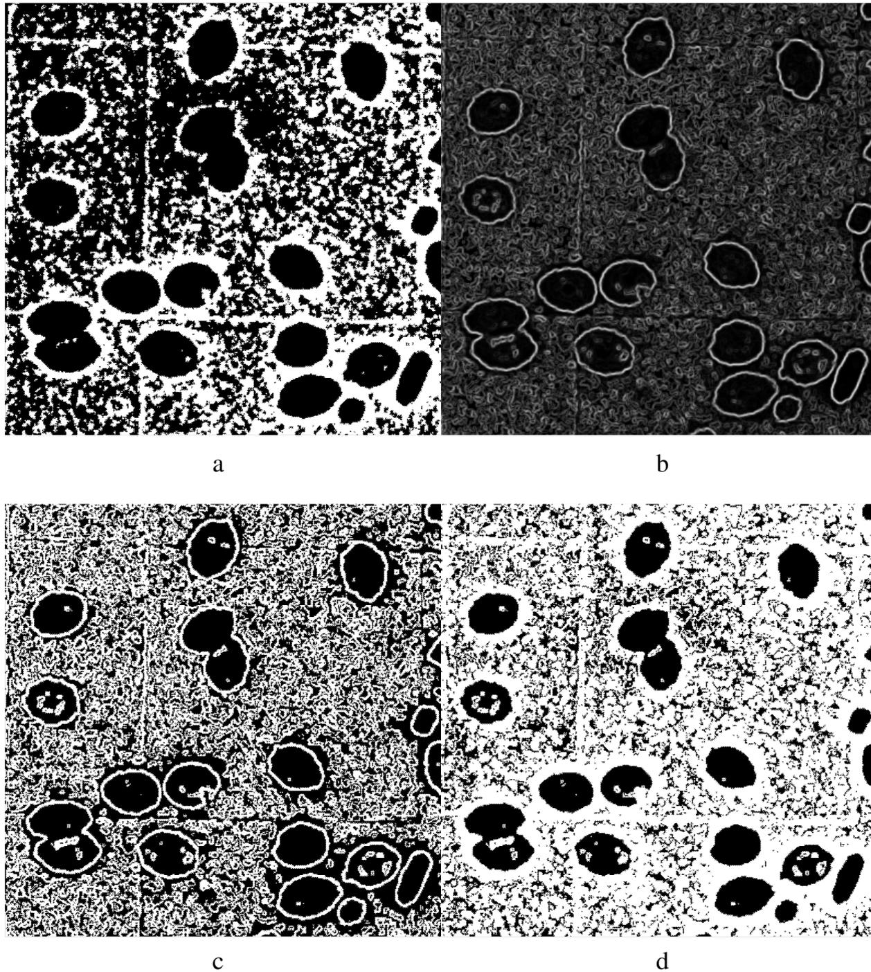
**Figure 4.** Binarization and filtering results, a) CoG Thresholding, b) Sobel filter c) Otsu thresholding of Sobel filter, d) Logic Or.
