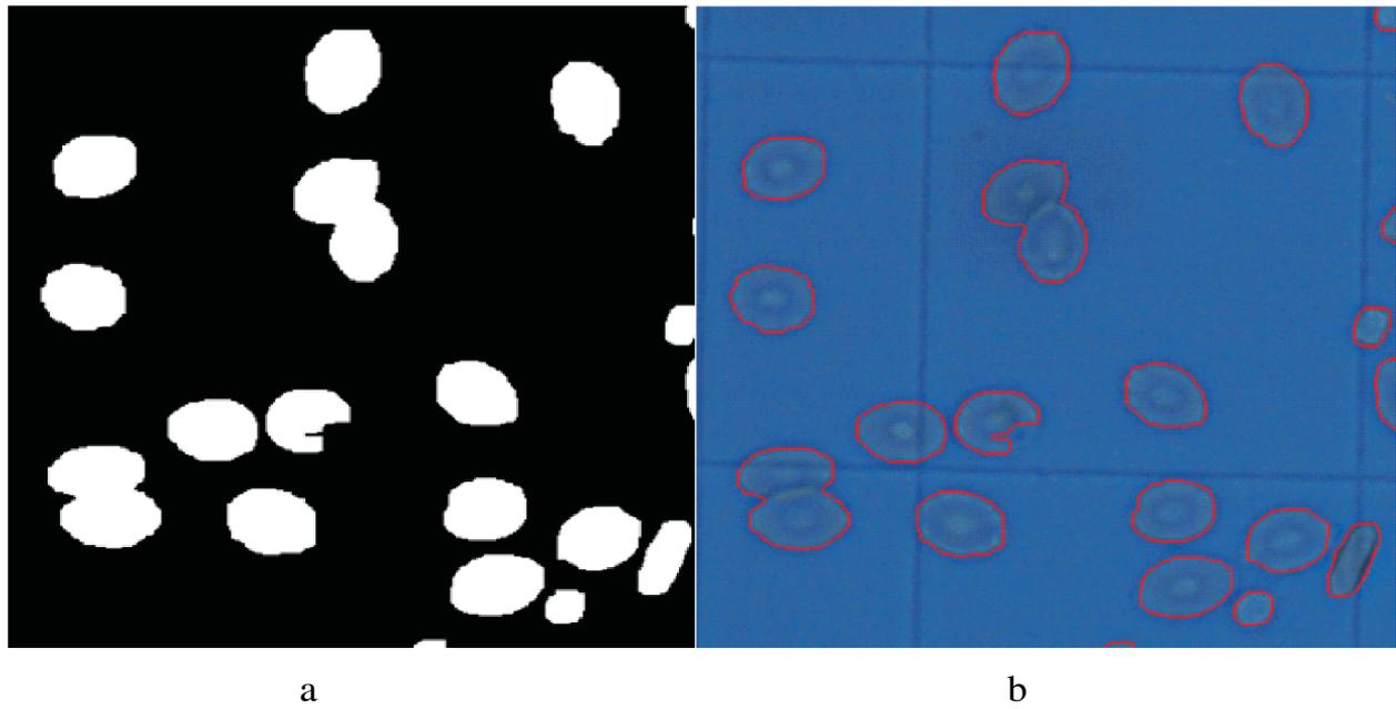
**Figure 6.** Detecting object borders, a) Morphological opening, b) Boundary detecting.
