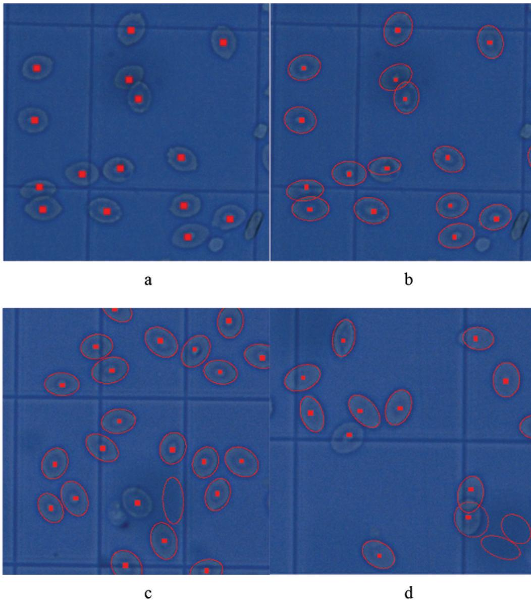
**Figure 9.** Manual marking and comparison results a) result of manual marking b-d) Manual marking and algorithm results.
