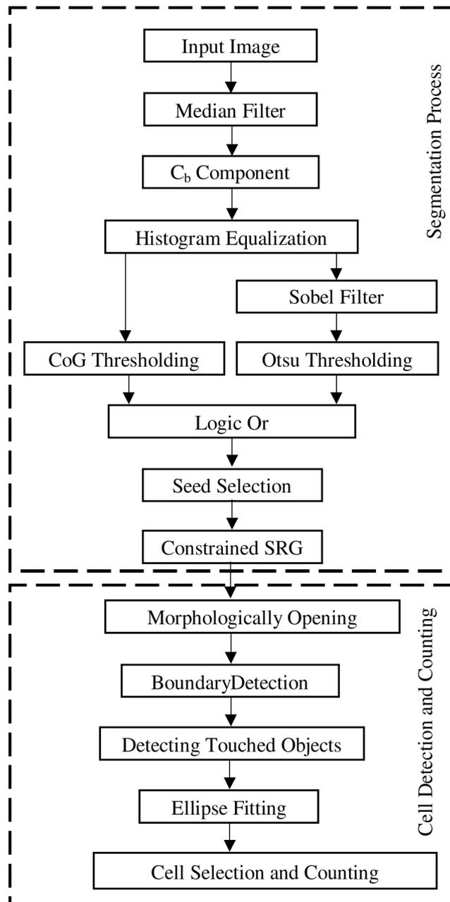
**Figure 2.** Block diagram of cell detection and counting.
