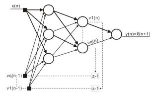
Figure 2. Network with recurrent hidden layer
