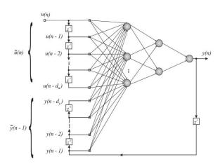
Figure 3. NARX network (Source [3]) with input and output delays
