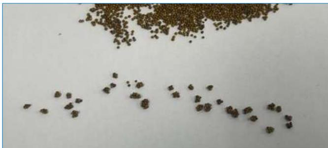
Fig. 5. 20/40 RCP proppants (dry) tested at conditions: 700 psi, 250 °F, 3.5 hours
