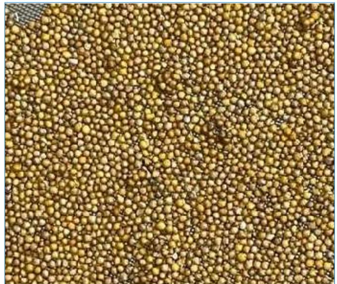
Fig. 3. 20/40 RCP proppants (wet) tested at conditions: 200 psi, 250 °F, 3.5 hours
