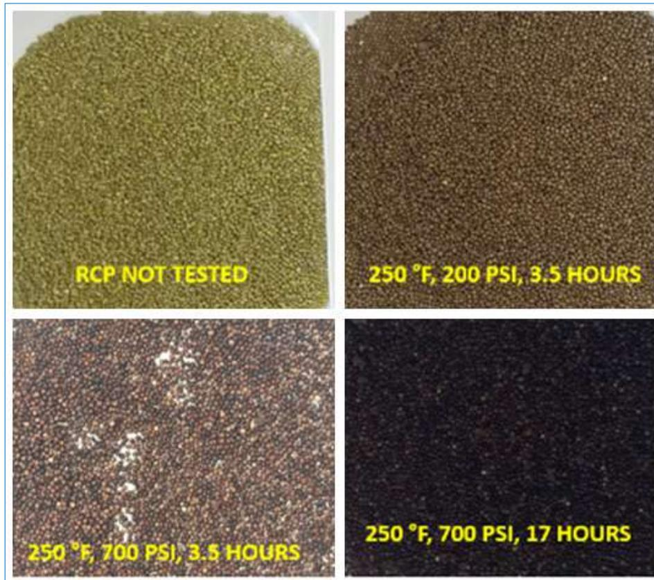
Fig. 8. Comparison among tested samples and original samples
