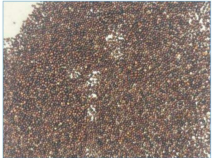
Fig.6. 20/40 RCP proppants (dry) tested at conditions: 700 psi, 250 °F, 17 hours
