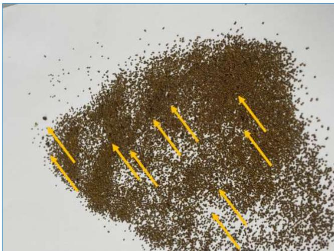
Fig. 4. 20/40 RCP proppants (dry) tested at conditions: 200 psi, 250 °F, 3.5 hours
