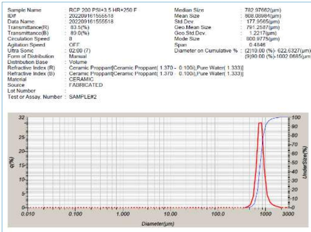
Fig. 9. Sample results of PSD analyzer
