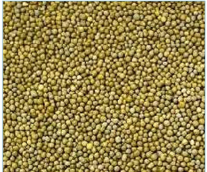
Fig. 2. 20/40 RCP proppants before any tests performed
