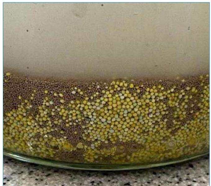
Fig. 7. Fluid sample taken during hydraulic fracturing treatment in the field
