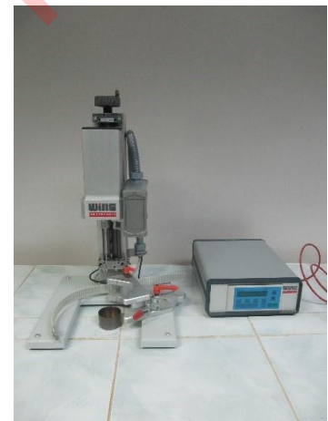
Figure 4. Miniature vane shear test device.
