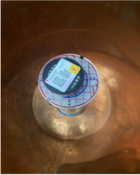
Figure 1. An experimental set-up of charcoal cartridges.
